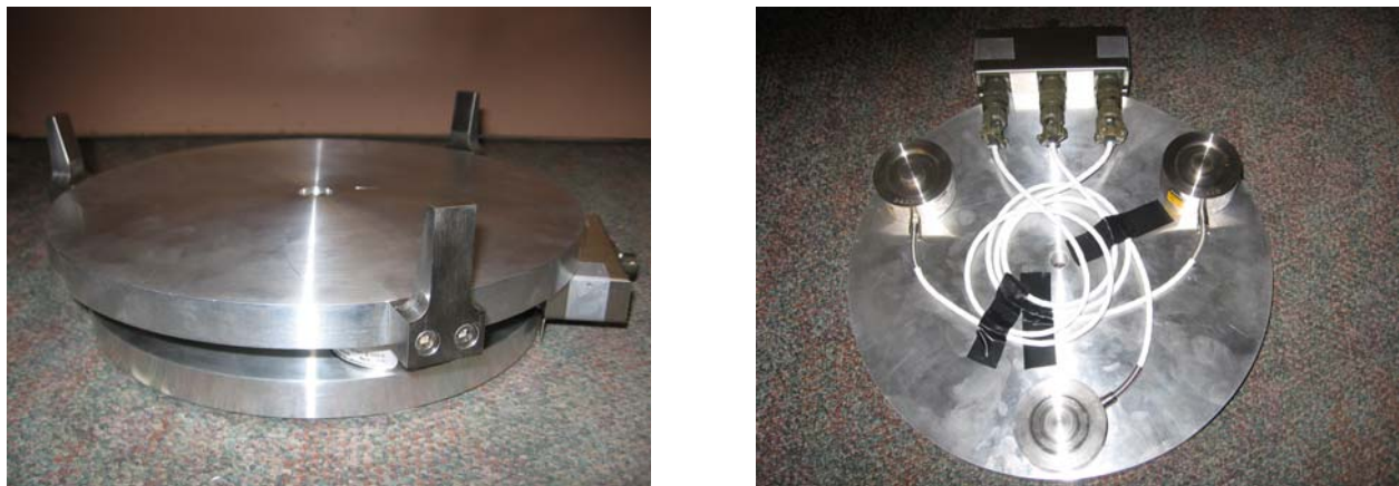
Figure 2. High-capacity load cell.
