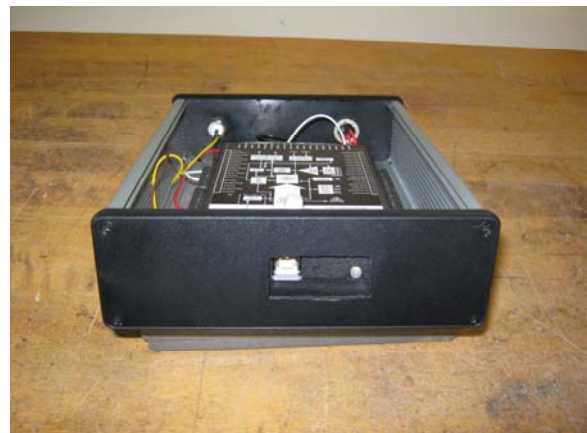
Figure 3. Protective box for DAQ board (cover removed).
