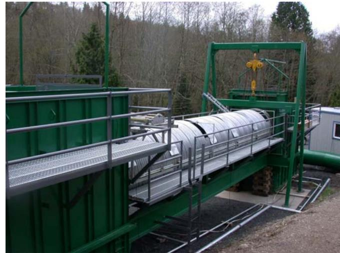
**TEST BED:** At the request of WSDOT, PNNL and Montgomery Watson Harza (MWH) have designed a test bed to identify the culvert designs and associated hydraulic conditions that allow successful upstream movement of juvenile salmonids at different life stages. The test bed is installed and has capabilities to
