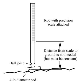
Figure 41. Rod and level with a large foot pad.<sup>(71)</sup>
