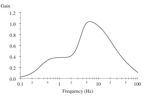
Figure 2. Weighting curve for human response to vertical vibration.
