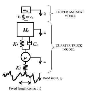
Figure 8. Prem model of truck response to road roughness.<sup>(12)</sup>
