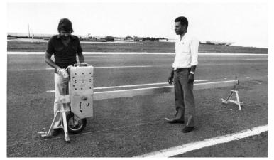
Figure 40. The TRRL Beam at the IRRE.<sup>(67)</sup>
