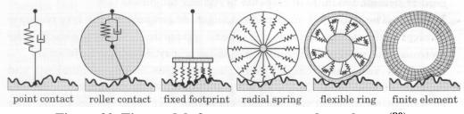
Figure 32. Tire models for response to road roughness.<sup>(80)</sup>
