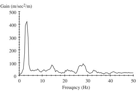
Figure 7. NRCC test vehicle transfer function.<sup>(39)</sup>
