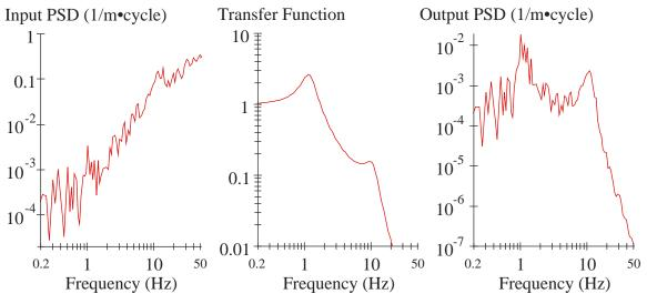
Figure 1. Passenger car suspension isolation.
