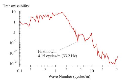
Figure 36. Road to spindle transmissibility over an impulse at higher speed.
