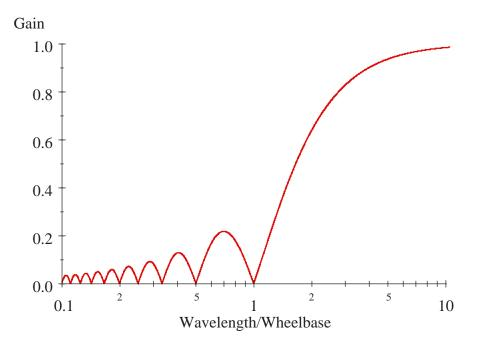
Figure 43. DipStick gain, small recording interval.
