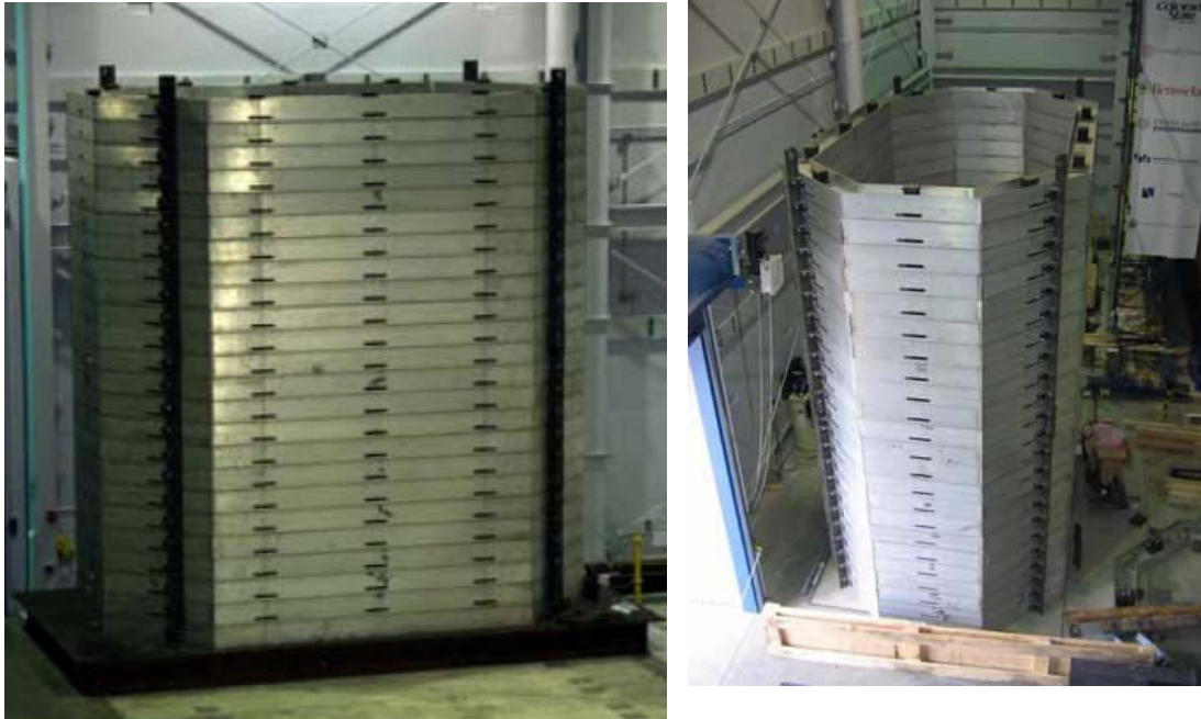
Fig. 3. Photographs of the stacked ring laminar shear box (24 ft high, 9 ft wide and
