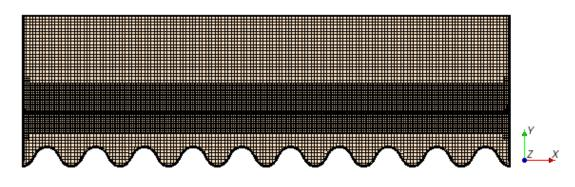
Figure 2.13 Cross sectional view of mesh scene along on a plane taken along the length of the increased section
