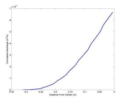
Figure 2.6: Cumulative discharge from the wall to the centerline in a cross-section of 6 inch water depth with symmetry boundary
