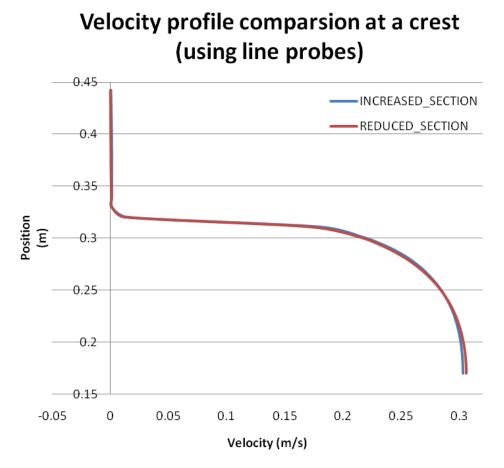
Figure 2.16 Velocity profiles for both reduced and increased sections at a crest
