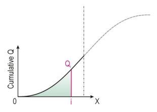
Figure 2.5: Cumulative discharge from the wall to the centerline
