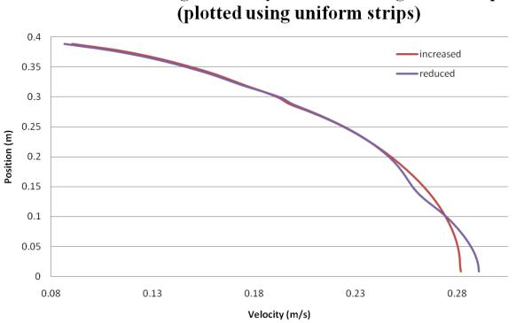
Surface-averaged velocity variation along the Crest plane (plotted using uniform strips)
