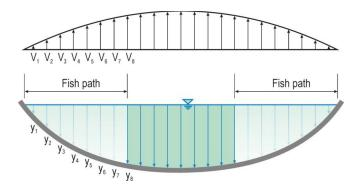
Figure 2.3: Flow path for the selected fish design criteria of velocity and depth
