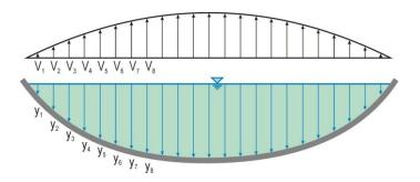
Figure 2.1: Variation of flow velocity and depth in a cross-section of a corrugated metal pipe
