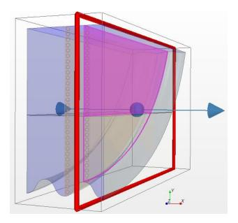
Figure 2.18 Cross sectional plane created at a crest in the porous region for a reduced section
