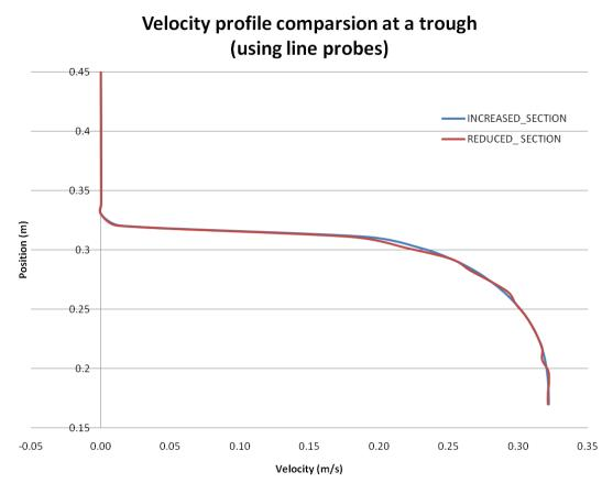
Figure 2.17 Velocity profiles for both reduced and increased sections at a trough
