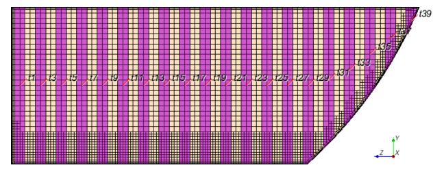
Figure 2.19 Representation of odd numbered Uniform strips of 1 cm width created along the fluid section
