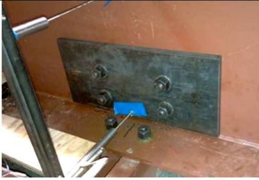
Fig. 3 View of backing plate on fascia side of girder web on Specimen 3
