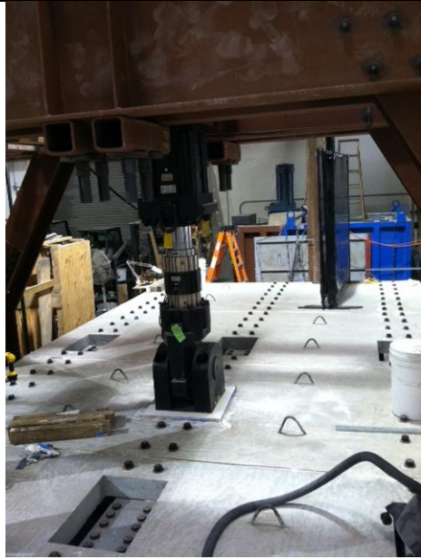
Fig. 1 View of top of bridge with actuator resting on load distribution plate
