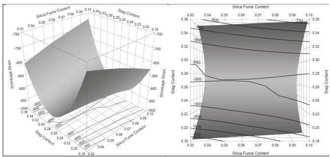
20 FIGURE 3 (a) response surface plot for series III (b) 2-D Contour plot
