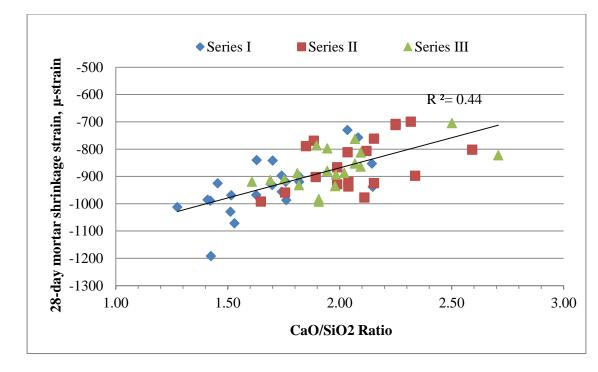
2 FIGURE 5 the relationship between Ca/Si ratio and 28-day shrinkage strain
