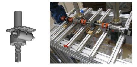
Figure 3 Screw jack driving system
