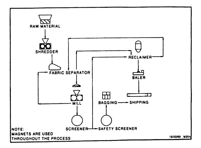
In the granulator process, steel cord and bead wire are removed and close tolerance-revolving steel plates are used to cut the scrap tires into granulated CRM. The granulated CRM is cubical, uniformly shaped with a low surface area with sizes ranging from 9.5 mm to 2.0 mm (3/8 inch to No. 10 sieve).
