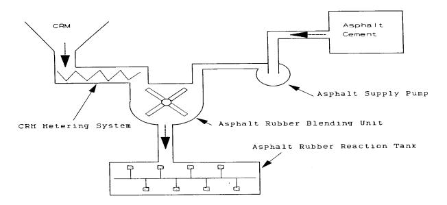
this theme. Any system used for blending asphalt rubber should be evaluated for its ability to produce a uniform, "reacted" product.
