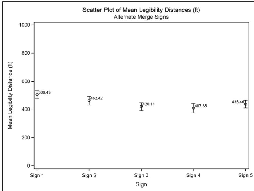
Figure 1. Legibility Results for Alternate Merge Sign Alternatives (95% CL about the mean shown)
