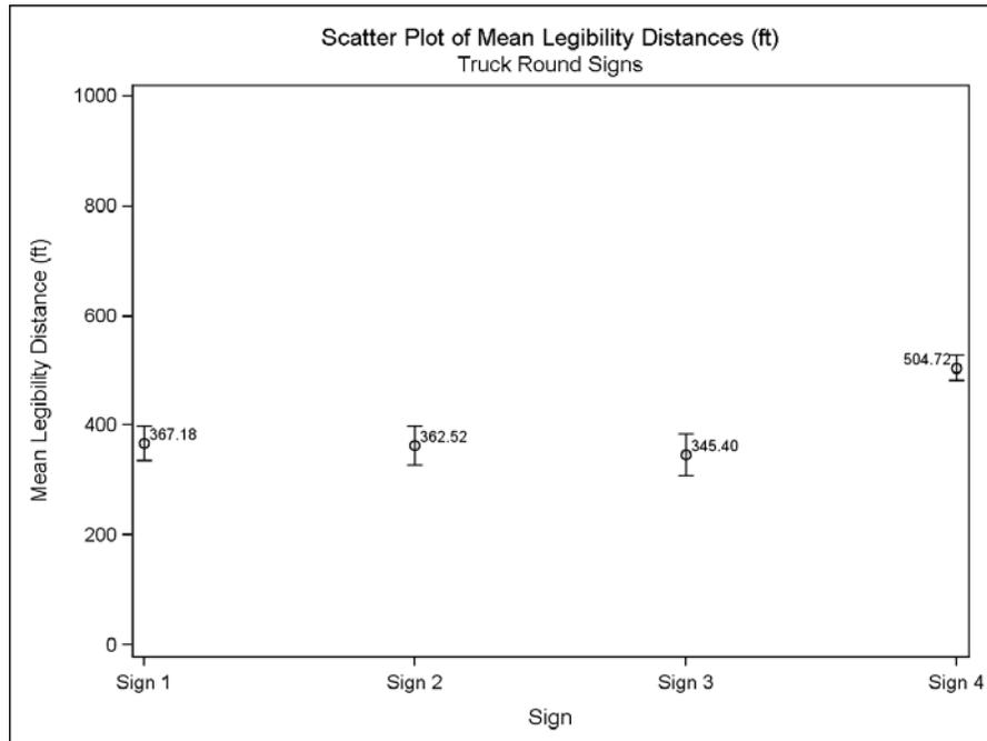
Figure 5. Legibility Results for Truck Roundabout Sign Alternatives (95% CL About the Mean Shown).
