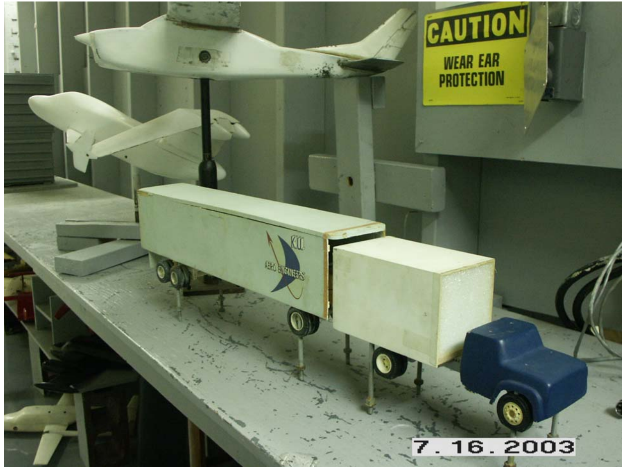
Figure 4. Model of Tractor-Trailer for Aerodynamic Data Collection.
