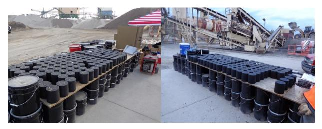
Figure C-12. Compacted samples of Intermediate and Surface layer
