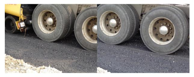
FigureC-10. Rutting of FRL due to weak DGAB
