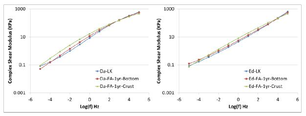
Figure 6. Complex shear modulus master curve at 64 °C for two sealants exposed to different aging conditions
