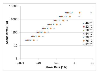
Figure 7. MSCR test results, shear stress vs. shear rate at various temperatures.
