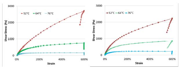
Figure 8. Shear stress vs. strain for two sealants at three different temperatures
