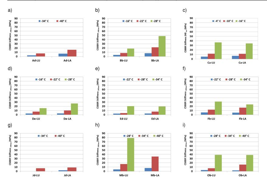
Figure 2. Effect of vacuum aging on CSBBR stiffness (@ 240s) at various temperatures.
