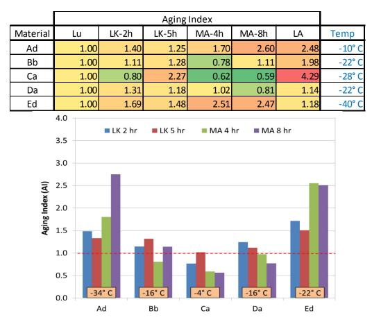
Figure 3. CSBBR sealant stiffness results illustrating the effect of various aging mechanisms
