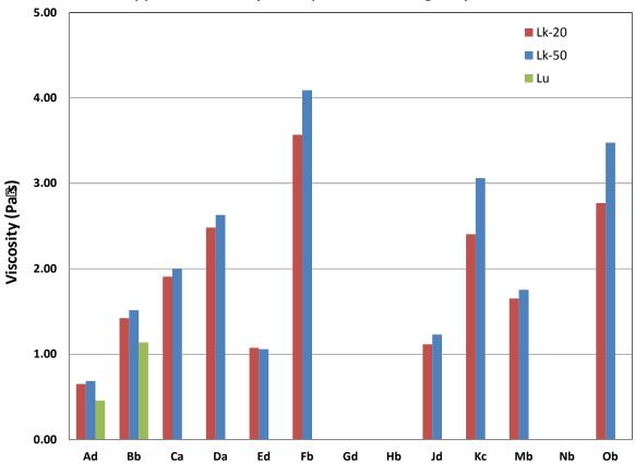
Apparent Viscosity at 60rpm for Kettle Aged Specimens
