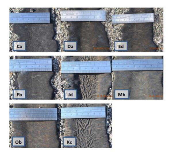
Figure 4. Pictures taken from routed and sealed cracks at ATREL test site to illustrate surface aging of various sealants under same weathering conditions without vehicular loading.
