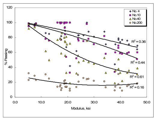
Figure 19. Grain size distribution versus subgrade modulus for coarse-grained soils (1 ksi = 6.89 MPa)
