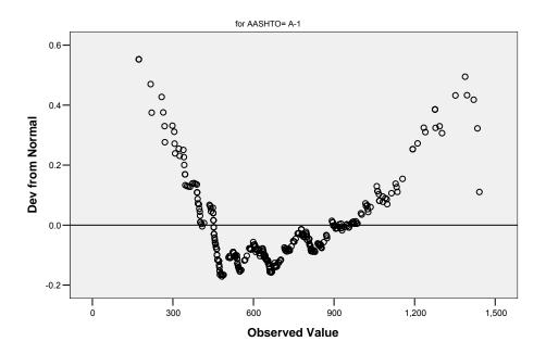
Figure 5. Detrended Q-Q plot of deflection data for A-1 soils (observed value of deflection in  $\mu m$ )
