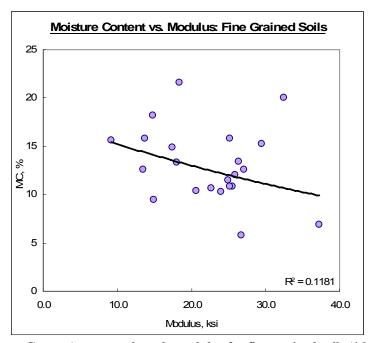
Figure 13. MC (Moisture Content) versus subgrade modulus for fine-grained soils (1 ksi = 6.89 MPa)
