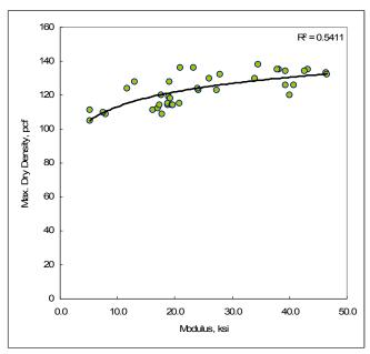
Figure 15. Maximum dry density versus subgrade modulus of coarse-grained soils (1 ksi = 6.89 MPa; 1 pcf =  $1 \text{ kg/m}^3$ )
