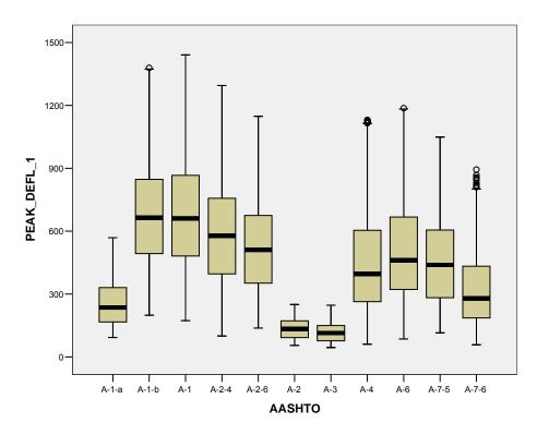
Figure 6. Box Plot of Deflection D1 (PEAK\_DEFL\_1) Data by Soil Type (deflection in μm)
