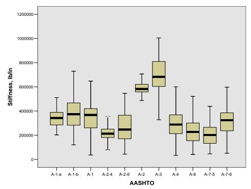
Figure 7. Box Plot of Calculated Subgrade Stiffness by Soil Types (100,000 lb/in = 17.5 MN/m)
