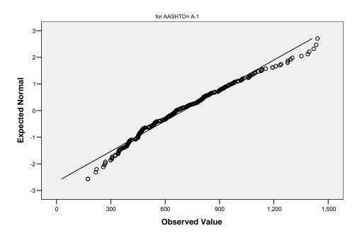
Figure 4. Q-Q plot of deflection data for A-1 soils (observed value of deflection in  $\mu m$ )
