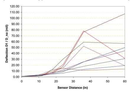
Figure 2. Type II Normalized Deflection Basin (1 in = 2.54 cm, 1 mil = 25.4  $\mu$ m)
