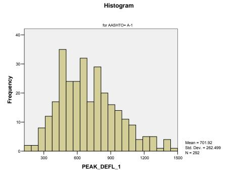
Figure 3. Histogram for deflection (PEAK\_DEFL\_1) data for A-1 soils (deflection in μm)
