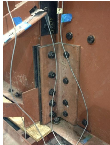
Figure 4: View of double angles used in most recent test trial of Specimen 3
