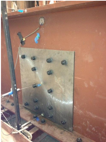
Figure 3: View of backing plate used in most recent test trial of Specimen 3
