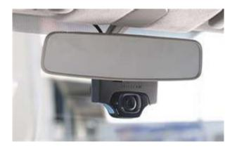
Figure 2. DriveCam Event-Triggered Video Data Recorder
