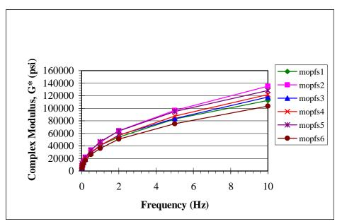
Figure 4 Frequency Sweep Results for Missouri Plant Mix Replicates (40°C)
