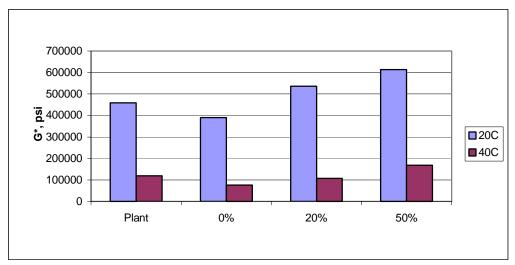
Figure 16 Summary of Complex Shear Moduli from Frequency Sweep at 10 Hz, Missouri
