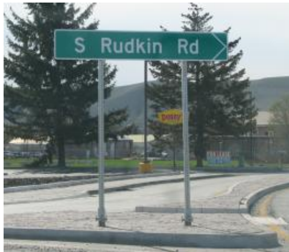
FIGURE 5.6 A Removable Sign on Roundabout Splitter Island
