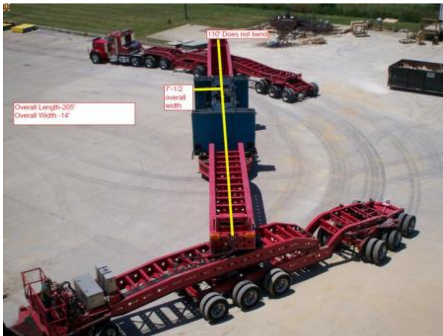
FIGURE 5.34 Turning Space Requirements of an OSOW Being Analyzed in a Parking Lot
