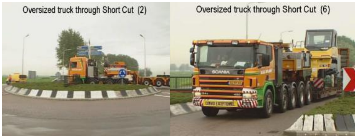
FIGURE 5.27 An OSOW Going through a Small Roundabout in the Netherlands
