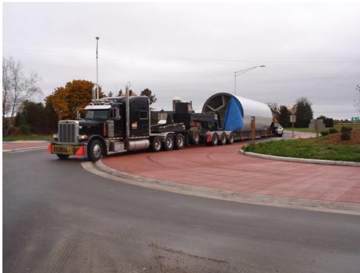
FIGURE 5.11 Advantage of Wide Truck Apron in Arizona
