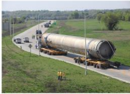
FIGURE 5.31 531,000 Pound, 210.5 Foot Long, Round Abatement Tower Approaching the Roundabout at Fredonia, Kansas
