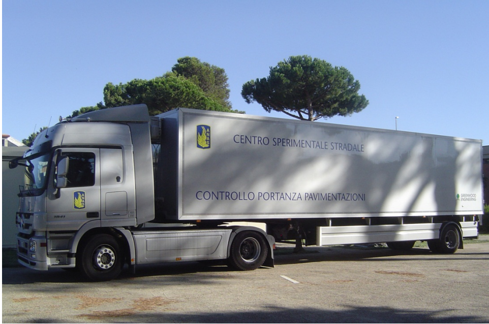
Traffic Speed Deflectometer (Owner - ANAS, the Italian Roads and Motorways National Agency; Photo Courtesy – Greenwood Engineering)
