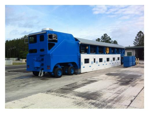
Figure 44. Insulated panels on HVS
