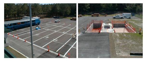
Figure 43. HVS Test tracks and test pits
