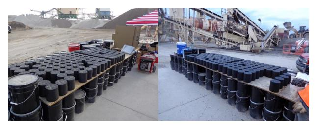
Figure 37. Compacted samples of intermediate and surface layers
