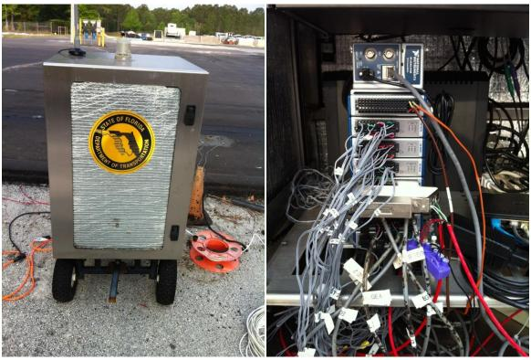
Figure 48. Mobile DAQ system
