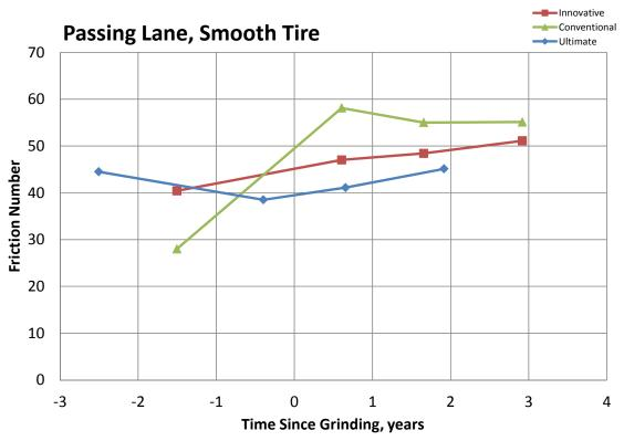
Figure 17. Friction Test – Passing Lane, Smooth Tire by Time Since Grinding.
