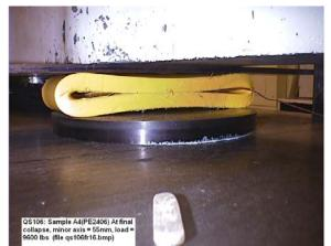
Figure 6-8 Sample at Near Flat State
