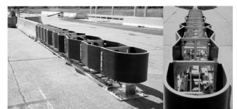
Figure 4-12 Hybrid Energy Absorbing Reusable Terminal (HEART<sup>TM</sup>) System
