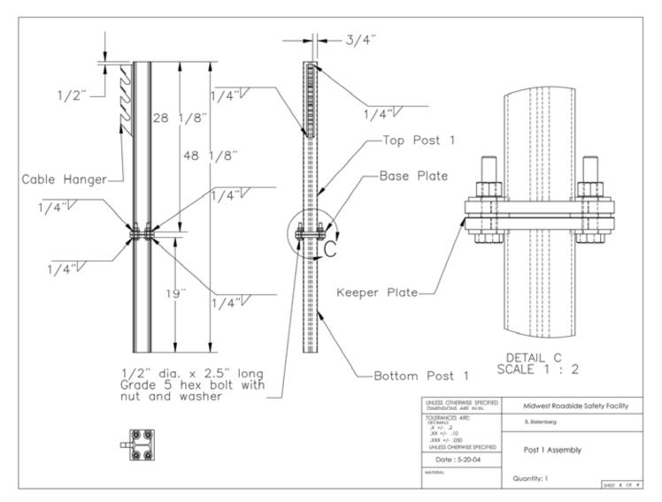
Figure 3. Modified NY Cable Anchorage Details
