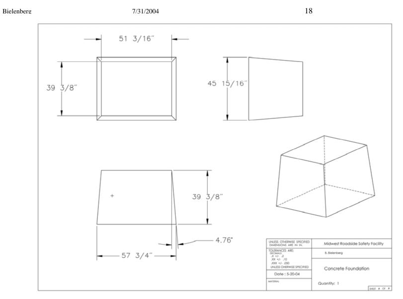
Figure 10. Modified NY Cable Anchorage Details
