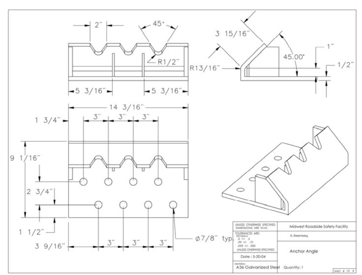
Figure 11. Modified NY Cable Anchorage Details
