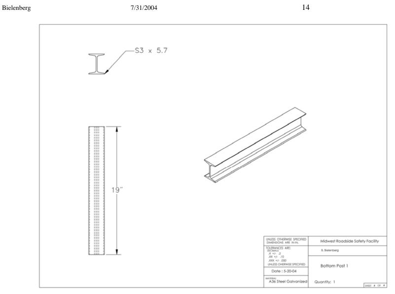
Figure 6. Modified NY Cable Anchorage Details
