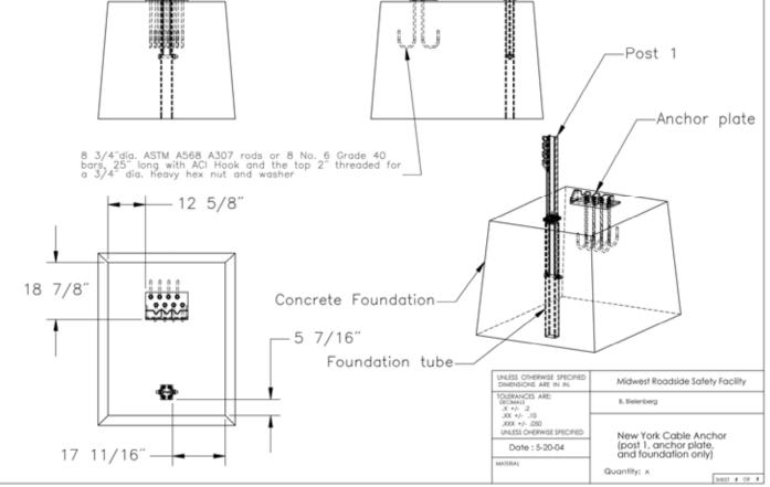
Figure 2. Modified NY Cable Anchorage Details
