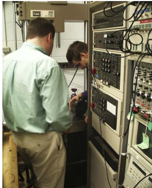
Figure 7 – Shaker table study to investigate frequency response of sensors. Left photo: Apparatus holding three LVDTs and two accelerometers symmetrically about the moving piston. Right photo: Control instrumentation with test frame in background.
