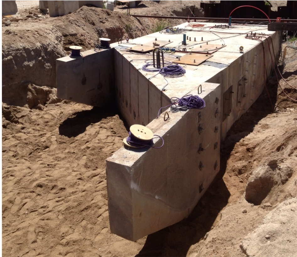
Figure 6. Photo of test setup and abutment geometry for 45° skew test.
