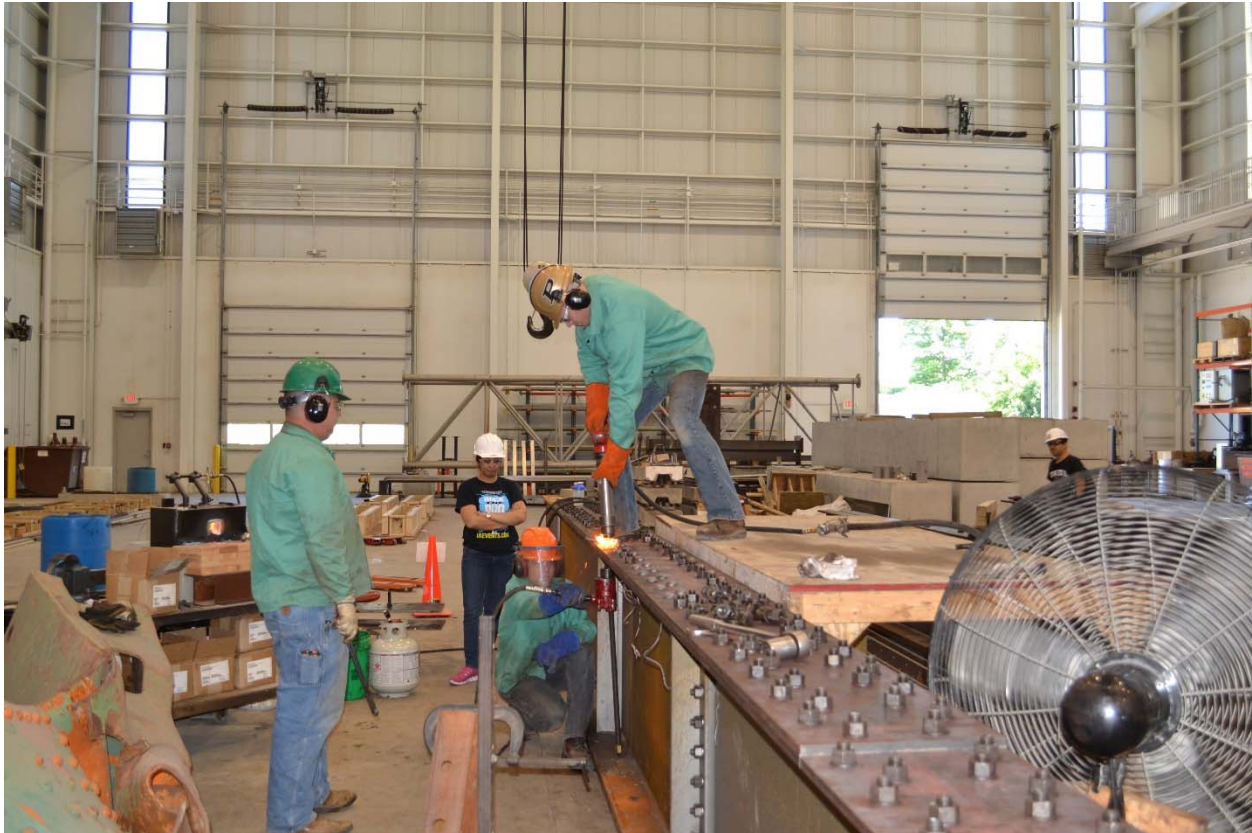
Figure 3: Specimen 36-3 fabrication - riveting cover plates to flange angles
