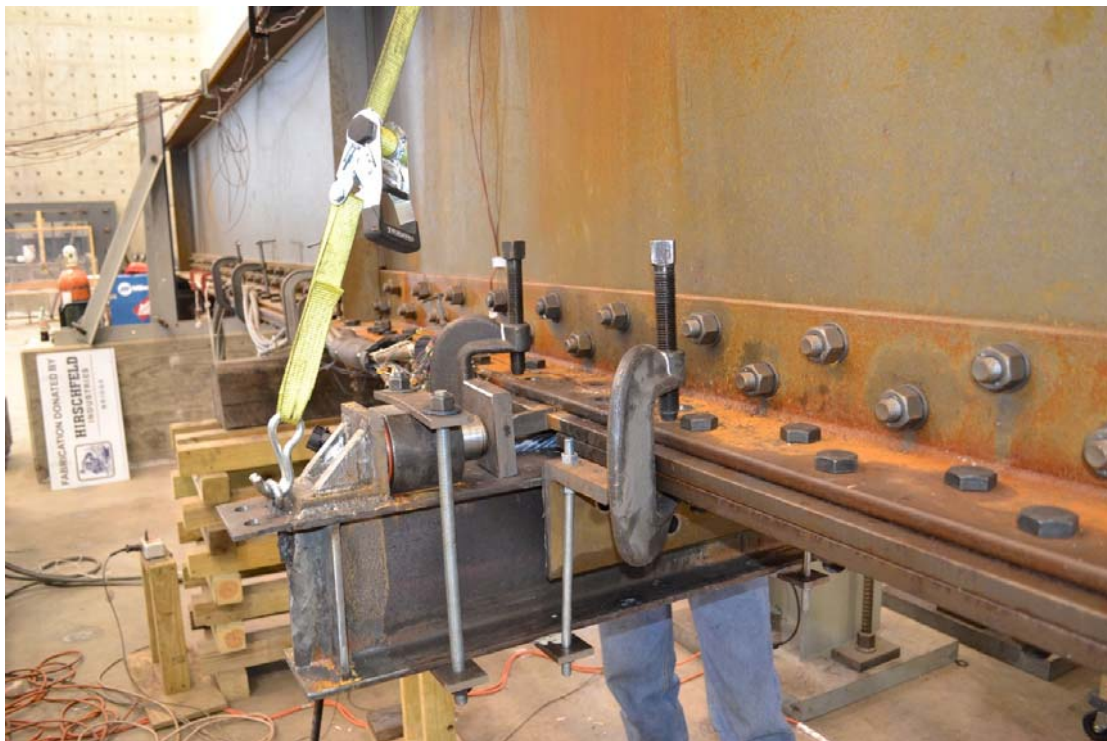
Figure 1: Specimen 36-2 with wedge driven into fractured upper cover plate
