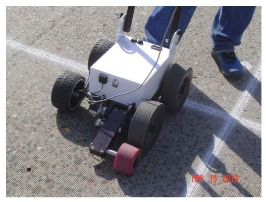
Figure B-2. SSI SC8800 Walking Profiler, close-up.
