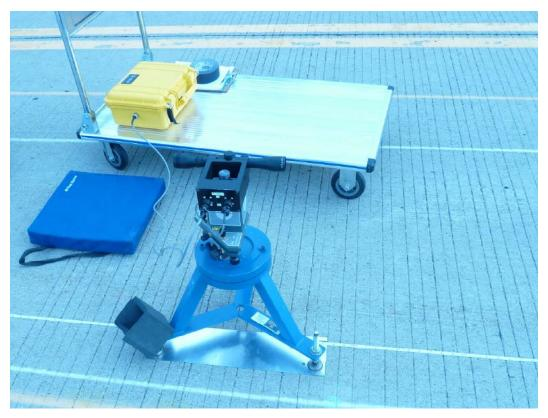
Figure B-13. Benchmark Profiler reference laser stand and power supply.
