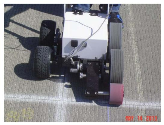
Figure B-4. SSI SC8800 Walking Profiler articulating arm.
