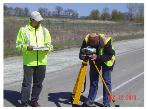
Figure B-14. Leica DNA 03 level.
