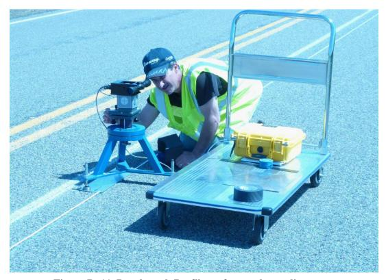
Figure B-11. Benchmark Profiler reference laser alignment.
