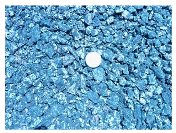
Figure A–6. Pervious hot mix asphalt texture.
