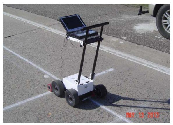
Figure B-1. SSI SC8800 Walking Profiler.
