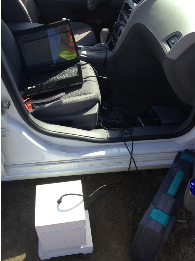
Figure 3. Test setup with sample and transducers in a wooden frame for stability
