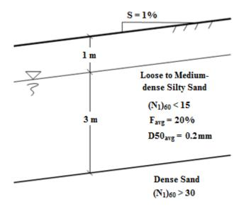
Figure 2-2 Soil profile used for the lateral spread displacement comparison study.
