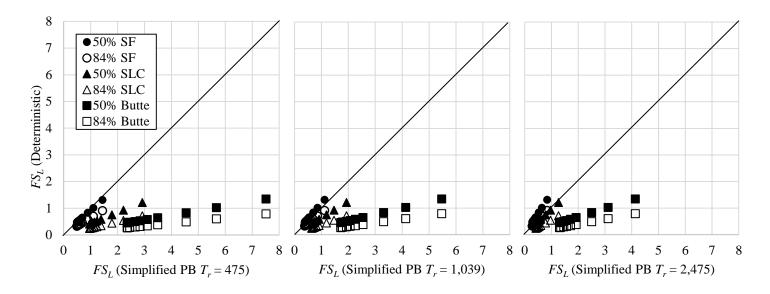
Figure 2-5 Comparison of deterministic and simplified performance-based values of FS<sub>L</sub>.
