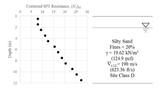
Figure 2-1 Soil profile used for the liquefaction initiation comparison study.
