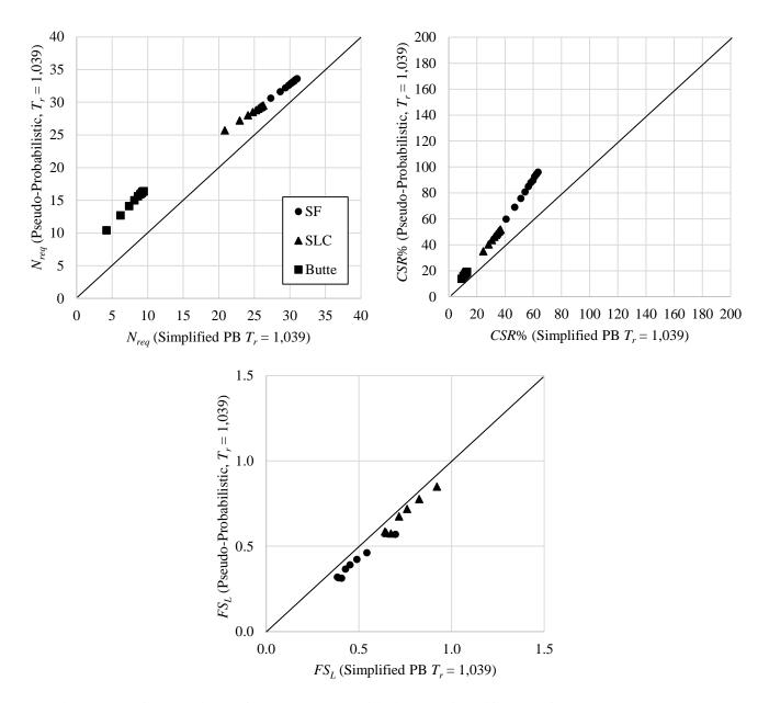
Figure 2-3 Comparison of pseudo-probabilistic and simplified performance-based values of  $N_{req}$ , CSR%, and FS<sub>L</sub>.
