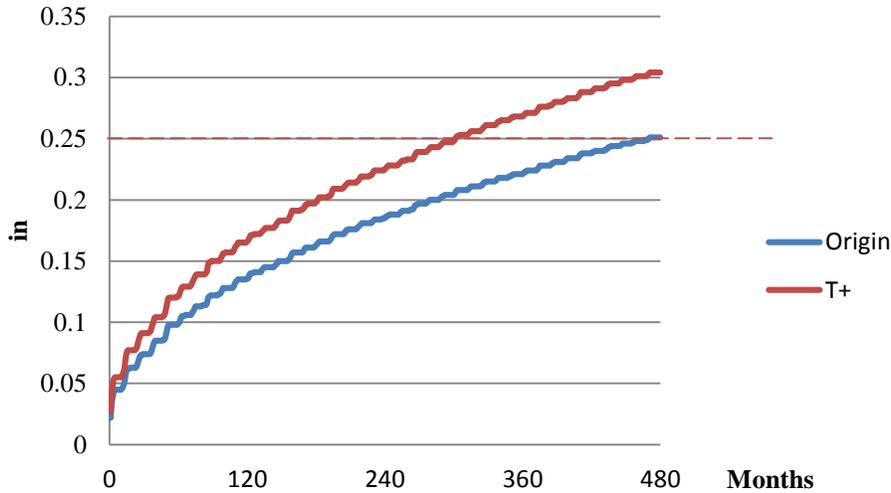
**FIGURE 4 Prediction of AC Rutting in Virginia.**
