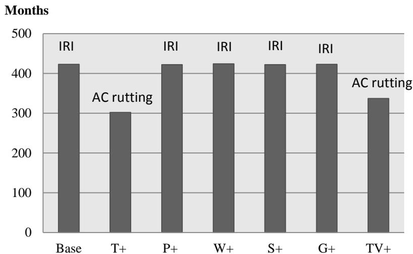
**FIGURE 3b Pavement Service Life, Virginia.** (*T* = temperature, *P* = precipitation, *W* = wind speed, *S* = percent sunshine, *G* = ground water level, and *TV* = temperature variation)
