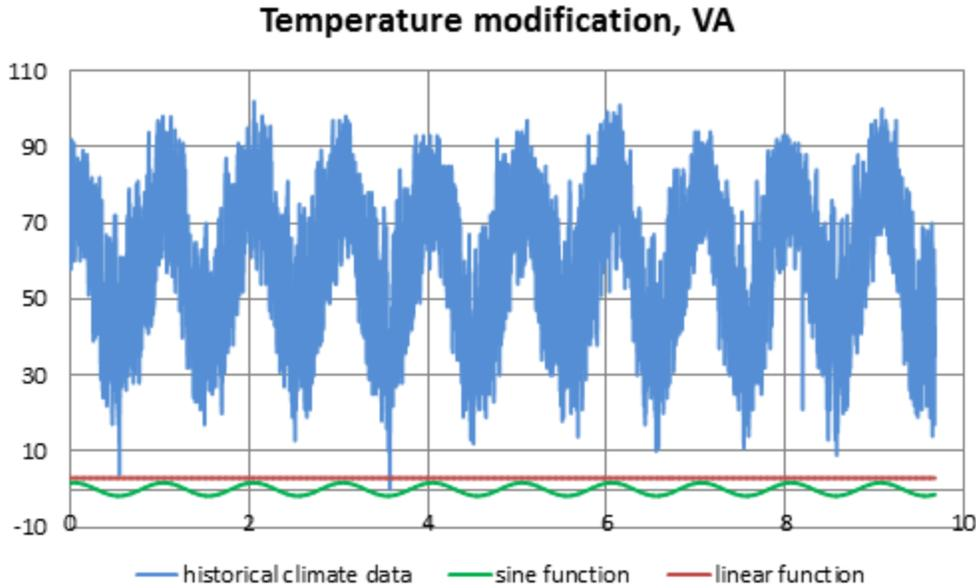
**Figure 1 Temperature modification for Richmond, VA. (Vertical axial: temperature (°F), horizontal axial: year.)**
