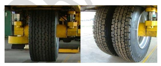
Figure 3-3. Test tires: WBT and DTA.
