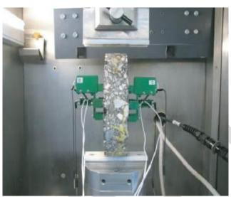
Figure E-6. Superpave IDT test setup.
