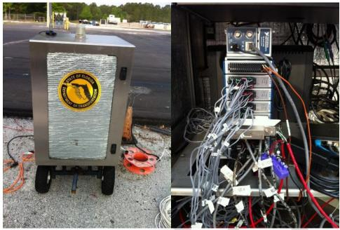
Figure E-10. Mobile DAQ system.
