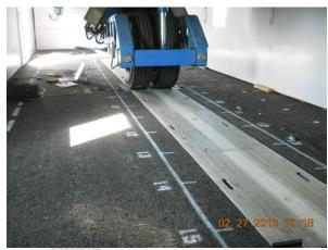
(b). Interior view of the temperature control chamber while validating HVS half-axle load
