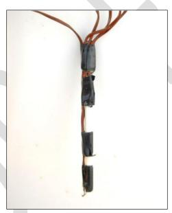
Figure F-15. Thermocouple tree with five Type-K thermocouples on a plastic dowel.
