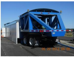
(a). Overall view of the HVS with temperature control chamber
