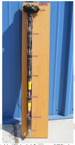
Figure F-22. A model multi-depth deflectometer (MDD), showing five modules.
