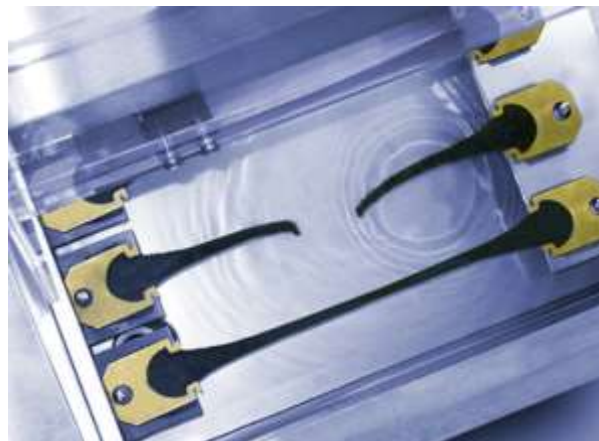
Figure 6- Image showing a ductility test in progress. Photo courtesy of Anton-Paar.
