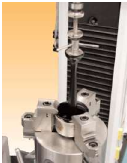
Figure 7- Toughness and Tenacity testing apparatus displaying a test in progress.
