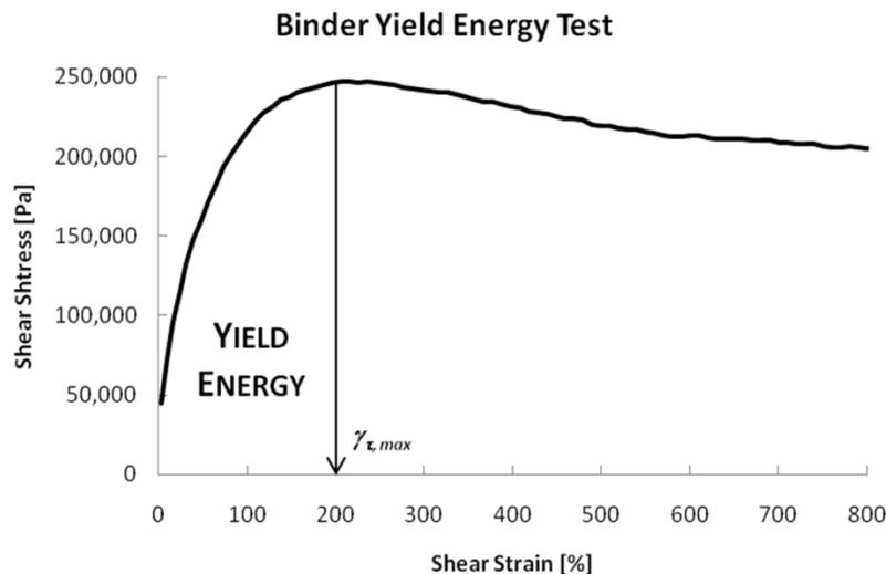
Figure 8. Typical output for BYET test
