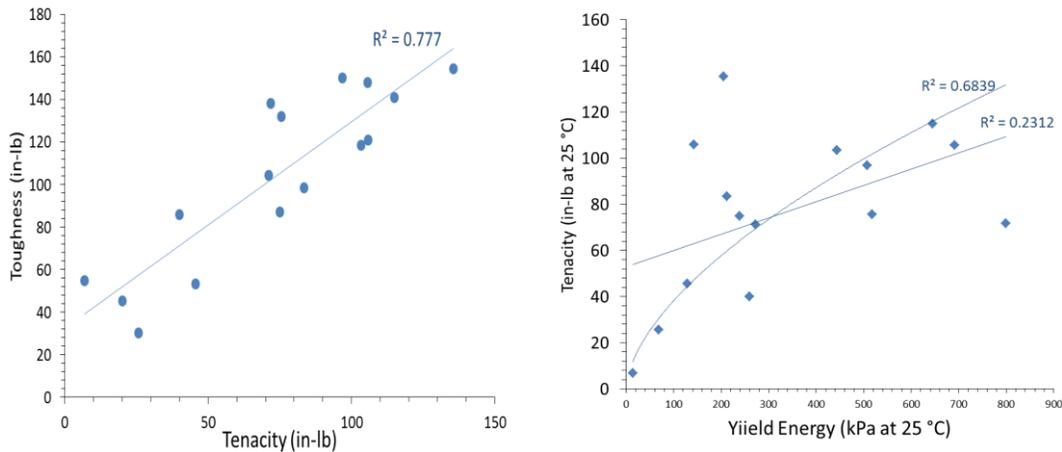
Figure 13. Toughness and tenacity for WCTG samples (left); Tenacity and yield energy at 25 °C (right)
