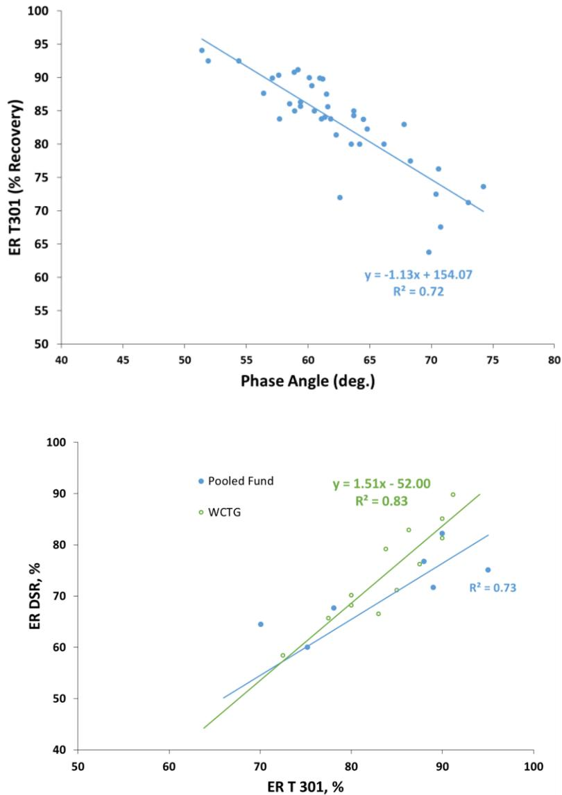
Figure 2. Correlation between T301 recovery and phase angle (top) and T301 recovery and ER DSR recovery (bottom).
