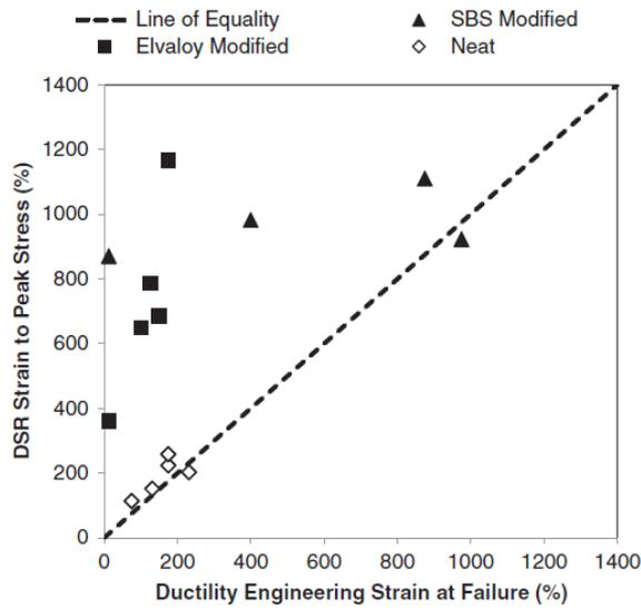
Figure 9. Comparison of BYET Strain at Peak Stress with T51 Strain at Failure [2].
