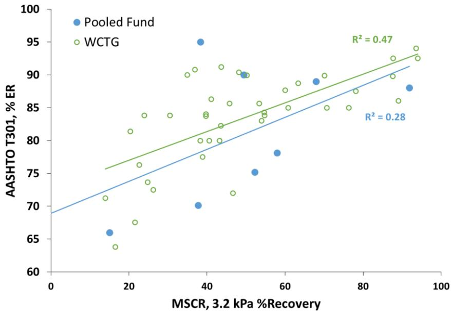
Figure 4. Correlation between ER T301 and MSCR %Recovery at 3.2 kPa for both Pooled fund and WCTG binders.
