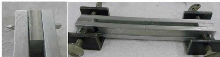
Figure 6.1. Photograph. Modified mold assembly for preparation of BBR-SENB beams.
