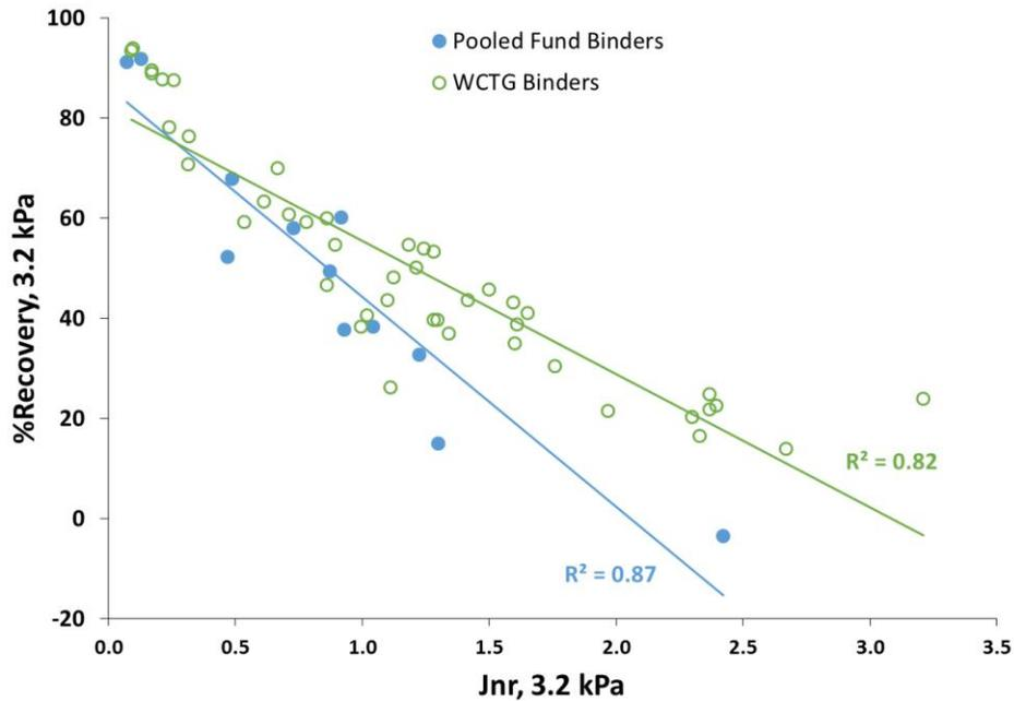
Figure 5. Jnr and % Recovery measured at 3.2 kPa.
