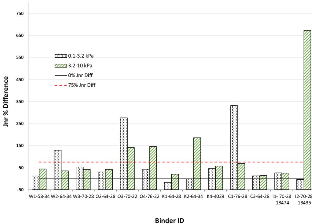
**Figure 7. %  $J_{nr}$  Diff values for each Pooled Fund binder. Where 0.1-3.2 kPa data represents the %  $J_{nr}$  Diff between stress levels of 0.1 and 3.2 and 3.2-10 kPa data represents the %  $J_{nr}$  Diff between stress levels of 3.2 and 10 kPa.**
