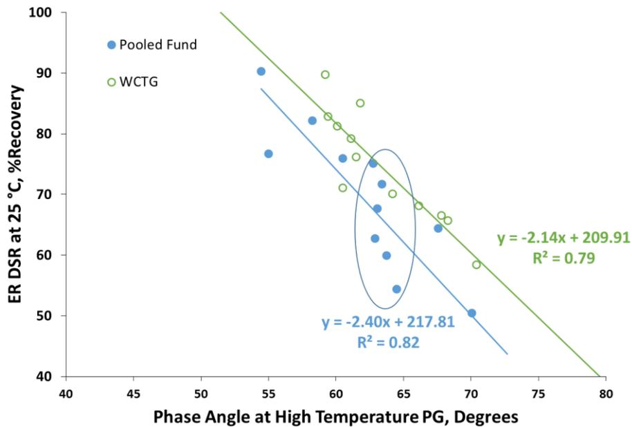
Figure 1. Correlation between Phase Angle and ER DSR results for the Pooled Fund and WCTG data sets.
