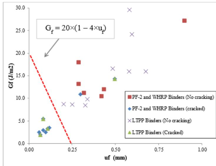
Figure 20. Proposed preliminary BBR-SENB specification based on RTFO aged conditions. Binders in the lower left triangle would fail the specification [8].
