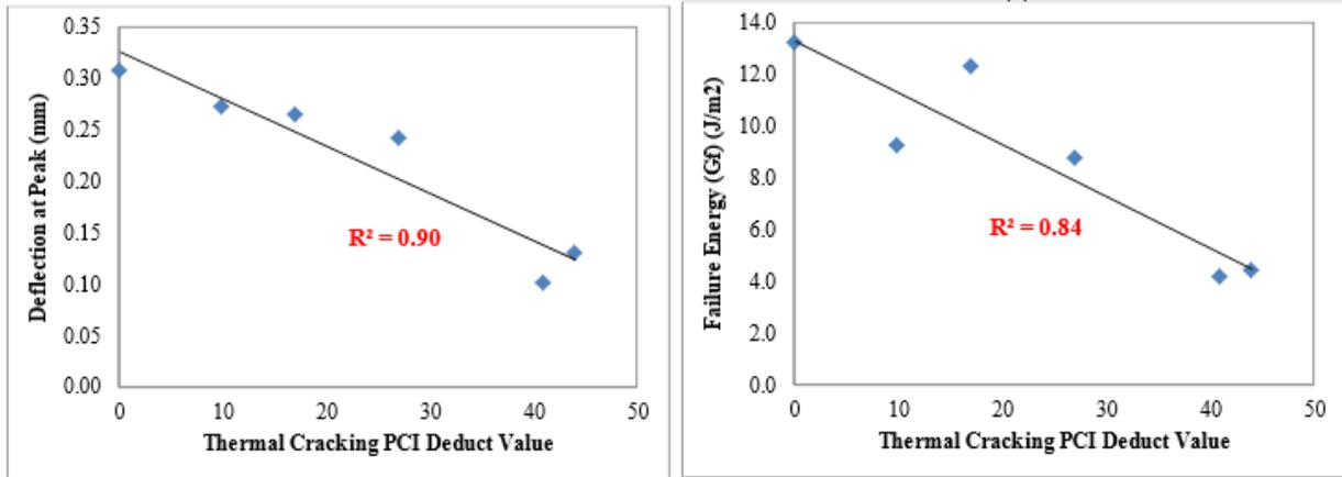
Figure 19. Correlation between deflection at peak load (left) and failure energy (right) with thermal cracking PCI deduct [8].
