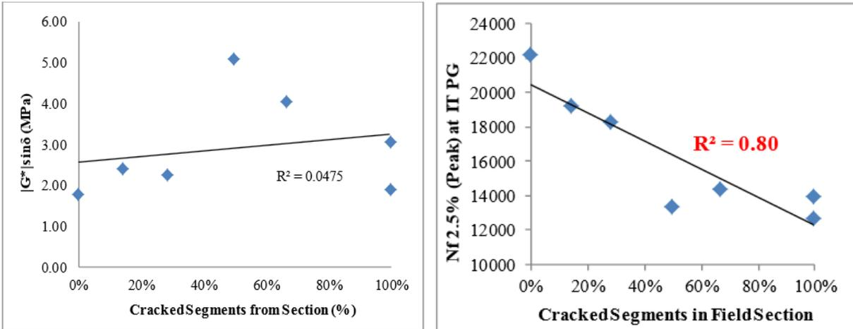
Figure 15. Comparison of Cycles to Failure Measured by LAS test to field fatigue cracking in Wisconsin [8].
