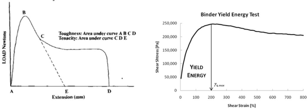
Figure 11. Definition of toughness, tenacity, and yield energy.
