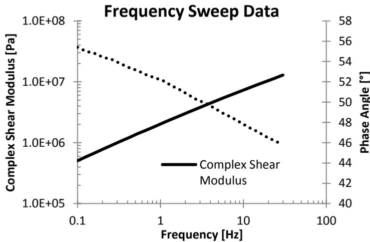
**Figure 1– Example output from frequency sweep test.**
