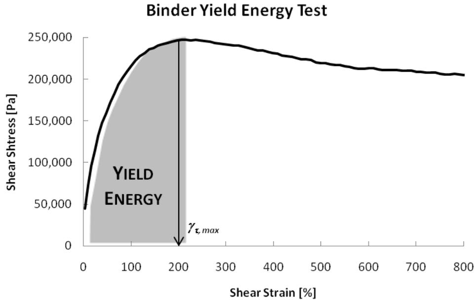
**FIGURE 7.1 – Visual representation of Binder Yield Energy Test parameters.**
