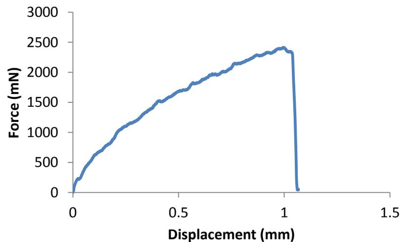
Figure 8.1. Graph. BBR-SENB typical force-displacement curve
