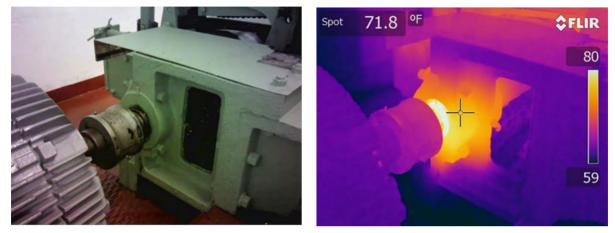
Figure 21: Standard and IR photos of Lewis and Clark River drawbridge mechanism (Astoria, Oregon)
