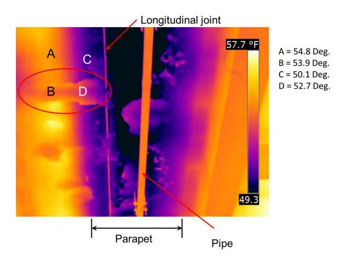
Figure 12: Thermal image of a deck soffit showing the conduction effect on the appearance of concrete delamination at the soffit
