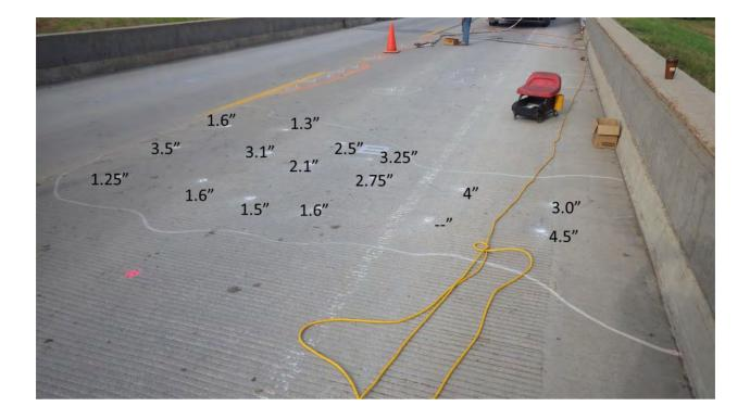
Figure 21: Drilled hole locations for borescope measurements
