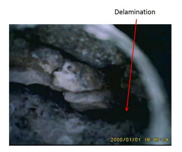
Figure 22: Borescope Image from location 6
