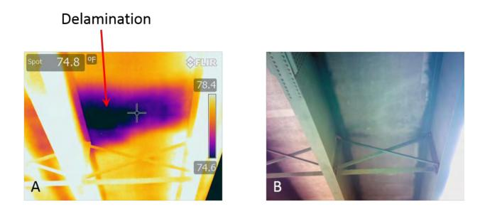
Figure 20: Infrared (A) and Digital (B) images from the soffit of the delamination in Figure
