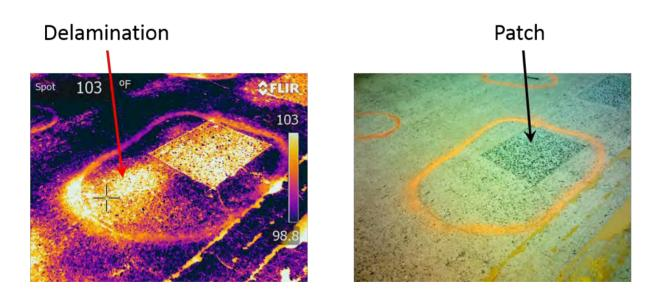
Figure 28: IR (A) and digital (B) images of a deck delamination over Ocmulgee River
