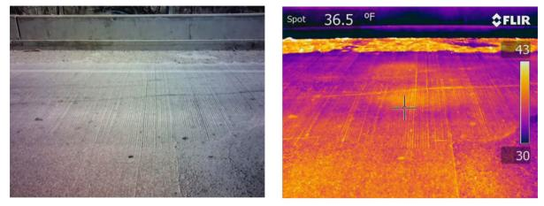
Figure 5: Standard and IR photos of bridge deck delamination (Vinton, Iowa)
