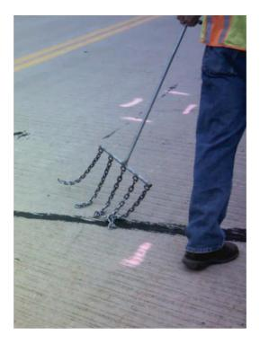
Figure 7: Chain drag used by MNDOT inspectors
