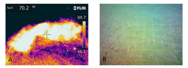
Figure 2: Infrared (A) and digital (B) images of a deck delamination in Kansas City
