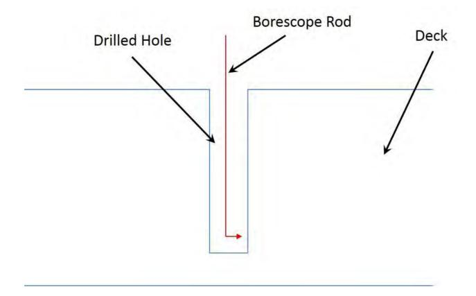
Figure 23: Schematic diagram of how the borescope is used
