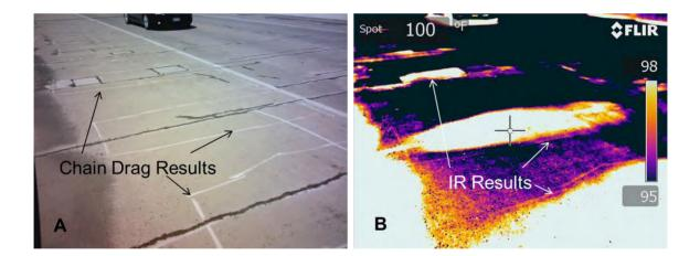
Figure 8: Chain dragging (A) and IR (B) results of deck delaminations.
