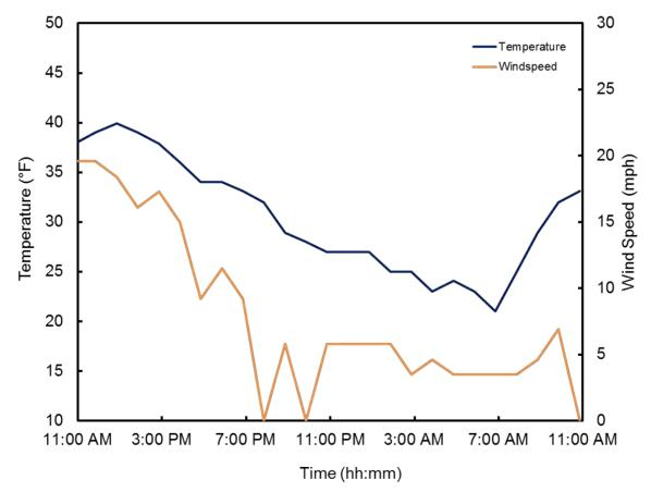
Figure 12: Weather data for the 24 hour period preceding IR inspection in Albany, New York
