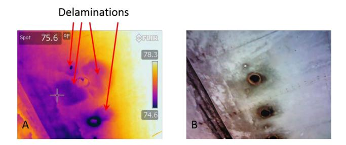
Figure 48: Morning infrared (A) and digital (B) images of a soffit delamination in Columbus, Ohio
