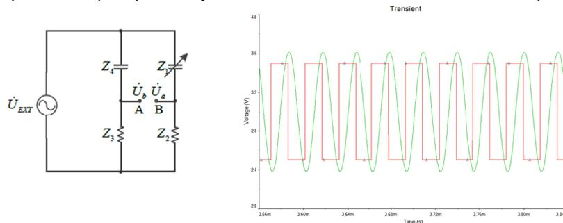
Fig. 3 The AC Wheatstone bridge and the waveforms used in C-Strain board.
