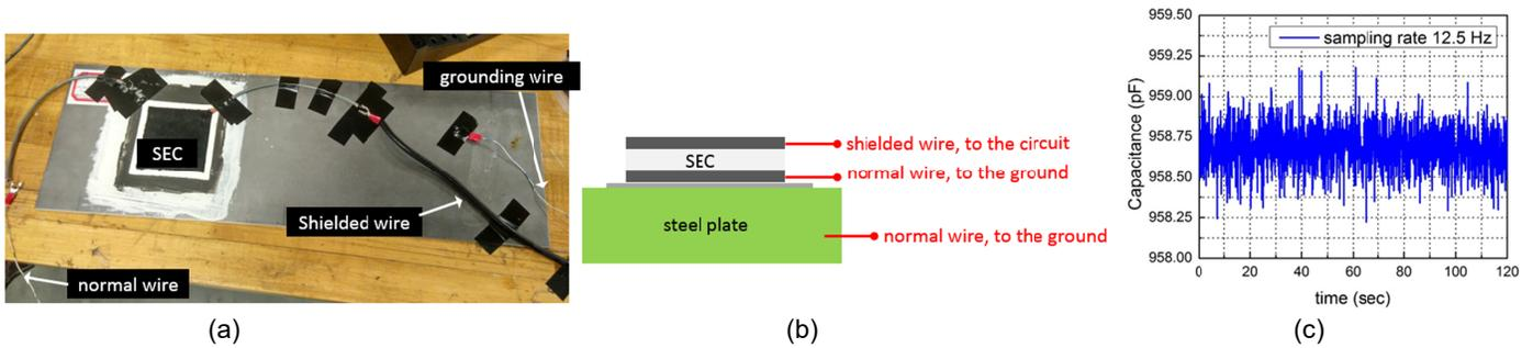
Fig. 9 (a) test setup; (b) schematic of sensor connections; and (c) a sample measurement
