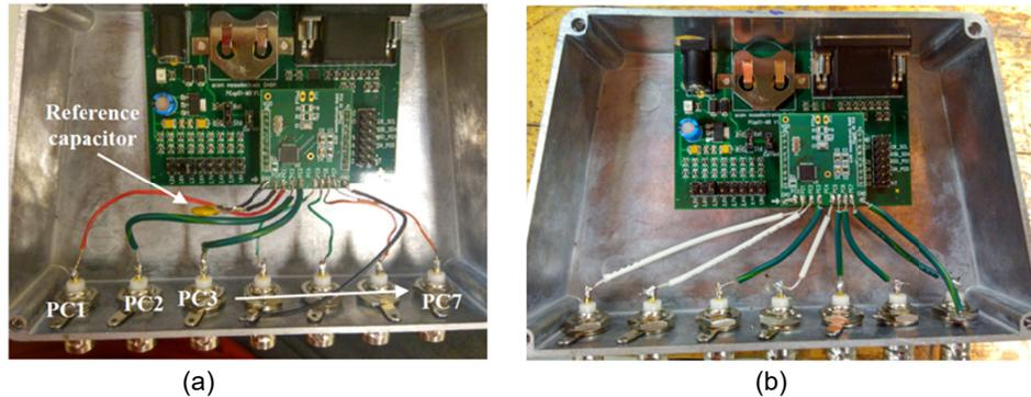
Fig. 8 (a) former and (b) updated DAQ setup with the PCAP02 board
