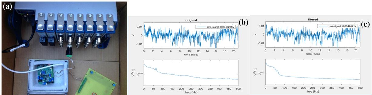
Fig. 7 Noise test for the C-strain sensor. (a) test setup; (b) the rms noise results; (c) the rms noise results with LPF applied.
