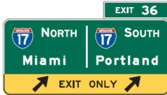
Figure 6 Example of signing for a two-lane exit ramp with two dropped lanes and a bifurcation beyond the mainline gore (MUTCD, 2009)
