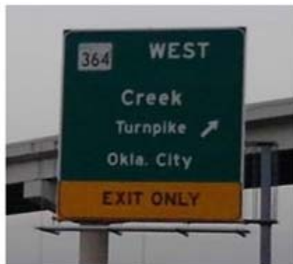
Guide Sign with Poor Legend Grouping Source: Jeremy Lance, Mid America Roads (unpublished data)
