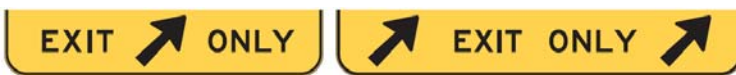
Figure 13 Example of arrow placement in EXIT ONLY panel in accordance with the MUTCD 2009.
