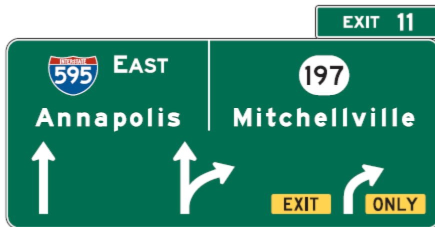
Figure 5 Overhead arrow-per-lane guide sign for a multi-lane exit with an option lane (MUTCD, 2009).
