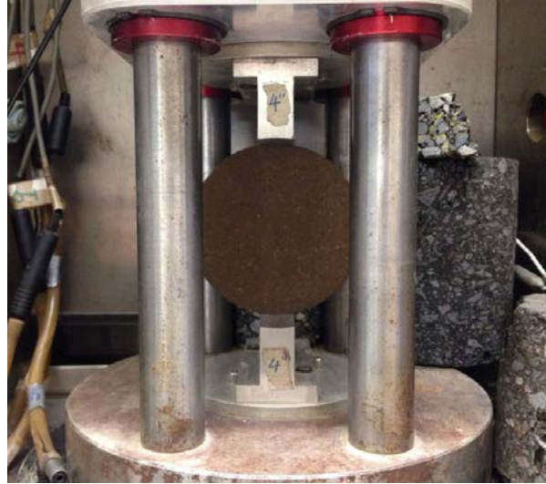
Figure 6.18: Indirect tensile test on GCTS
