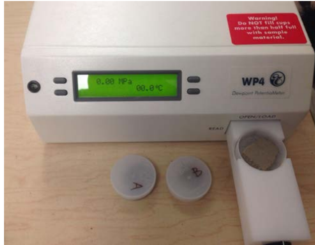
Figure 6.12: WP-4 Dewpoint Potentiometer device and specimens tested
