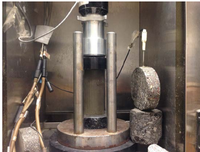
Figure 6.20: UCS sample and GCTS device
