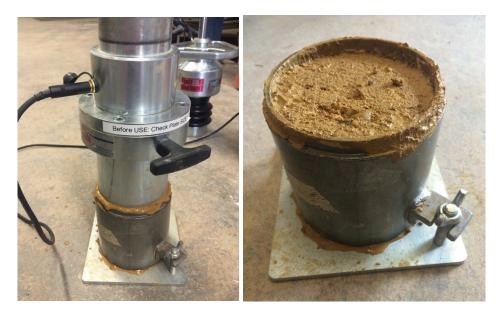
Figure 45- Permanent deformation and unleveled surface in the 4 inch mold after testing with Zorn LWD.
