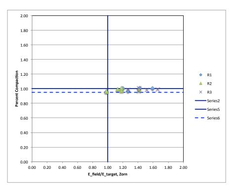
Figure 14- PC vs. Field to Target modulus ratio for Zorn LWD.
