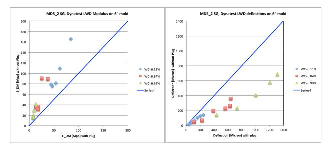
Figure 23. Measured modulus and deflection on 6 inch Proctor mold for Dynatest LWD with and without plug.
