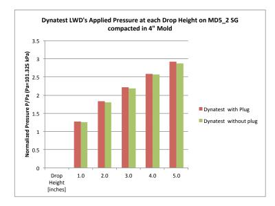
Figure 20- Applied pressure on 4 inch Proctor mold for Dynatest LWD with and without plug.
