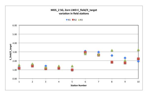
Figure 11- Measured field modulus to calculated target modulus ratio: Zorn LWD.
