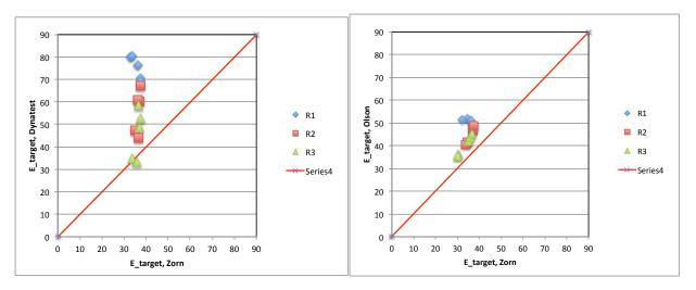
Figure 18- LWDs calculated Target modulus correlation.
