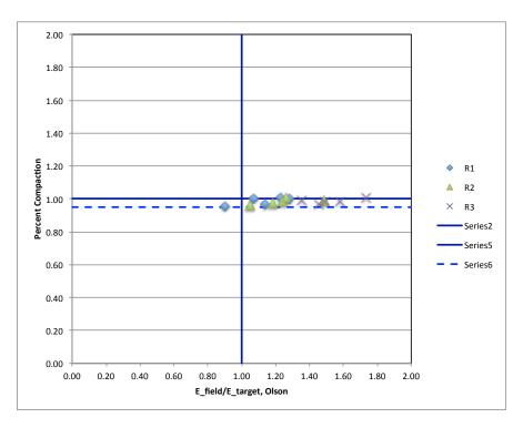
Figure 16- PC vs. Field to Target modulus ratio for Olson LWD.
