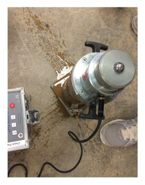
Figure 46- Water drained from sample compacted on wet side of OMC during LWD on Proctor mold testing.
