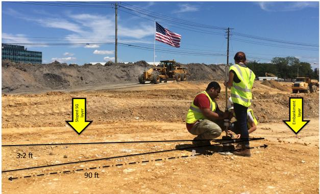
Figure 3- Maryland Route 5 LWD testing on Sloped Subgrade.
