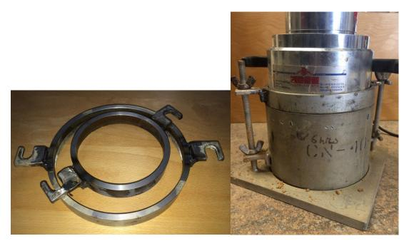
Figure 44- Collar designed for 4 inch and 6 inch molds.
