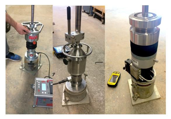
Figure 1- Zorn, Olson and Dynatest LWDs on 6 inch Proctor molds.
