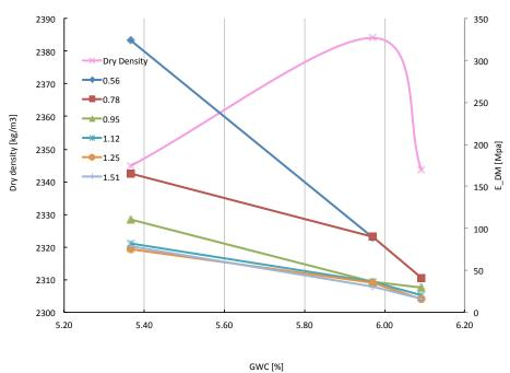
MD5\_2, Subgrade, Dynatest LWD Modulus without plug on 6" mold
