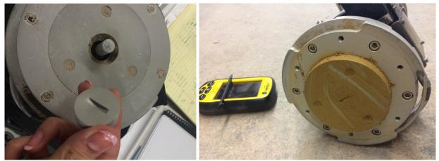
Figure 42- Dynatest Plugin to lock the center geophone for measurement of the plate deflection.
