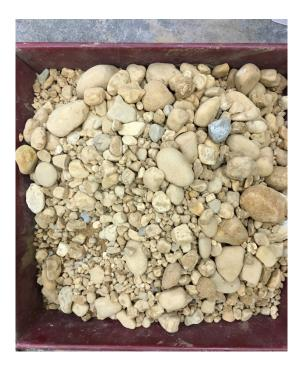
Figure 43- MD 5 Subgrade scalped coarse aggregate according to AASHTO T-99.
