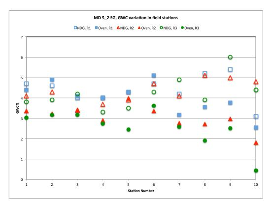
Figure 5- NDG and oven-dried MC measurements at each station for 3 rounds.
