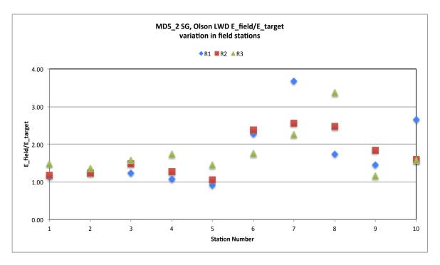
Figure 13- Measured field modulus to calculated target modulus ratio: Olson LWD.
