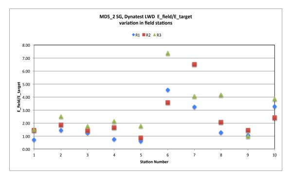
Figure 12- Measured field modulus to calculated target modulus ratio: Dynatest LWD.
