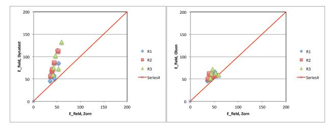
Figure 17- LWDs Field measured modulus correlation.
