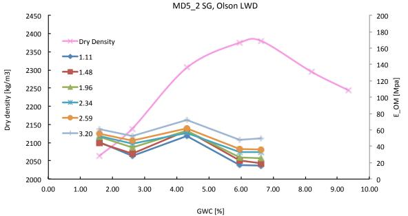
Figure 9- Olson LWD modulus on Proctor mold for different stress states (P/Pa) and Dry Density versus GWC.
