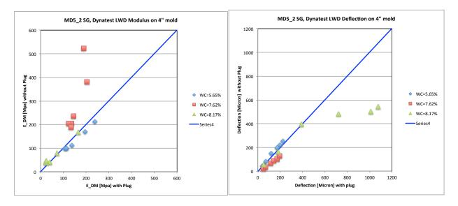
Figure 21. Measured modulus and deflection on 4 inch Proctor mold for Dynatest LWD with and without plug.
