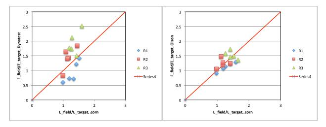
Figure 19- LWDs Field to Target modulus correlation.
