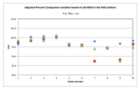
Figure 6- Percent compaction measured by NDG at each station for 3 rounds.
