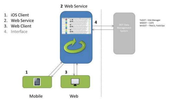
Figure 3: Illustration of the three software components of the HeadLight system
