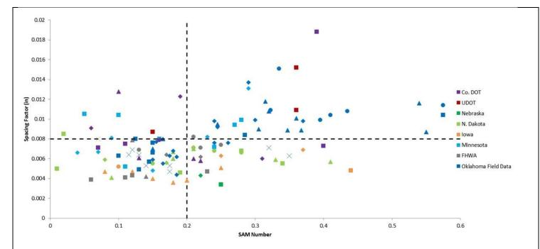
Figure 5 – Field testing data comparing the SAM number to the spacing factor for field mixtures from a number of different states with the spacing factor and SAM number compared.
