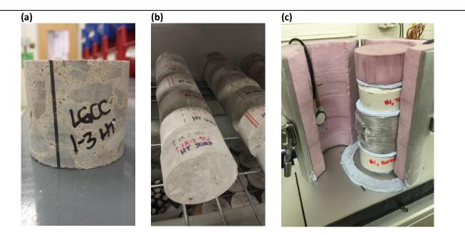
Figure 8 - Current Testing States (a) Sorption samples conditioning at 50% relative humidity (b) Sample labeling convention cut and cored LGCC sample (c) LGCC Test Setup.
