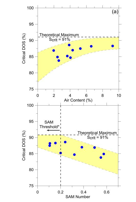
Figure 14 Projected Critical Degree of Saturation for Concrete Mixtures with a) Total Air Content and b) Air Quality (SAM Number) Using the Damage Index Following Three Freeze-Thaw Cycles
