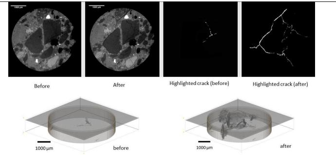
Figure 15 – An air entrained mortar sample shown both before and after a freeze thaw cycle. The highlighted cracks are shown from the cross sections. In addition, 3D data sets are shown of the crack distribution both before and after the freeze thaw cycle. The data was obtained with X-ray mCT.
