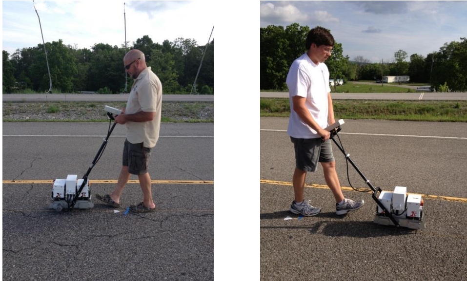
Figure 12 Reference profile measurements using the two SURPRO profilers.
