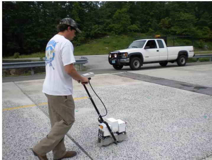
Figure 7. Reference profile measurements being taken with the SURPRO.
