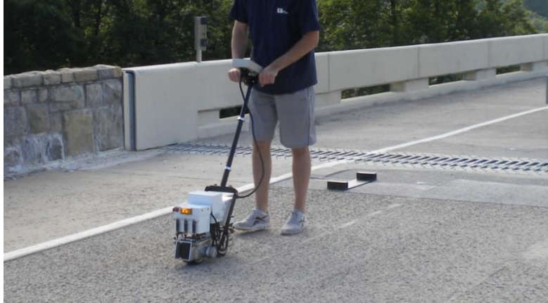
Figure 9 Reference profile measurements using the SURPRO.
