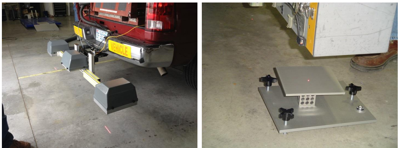
Figure 10 The Ro-Line lasers are displayed on the left and the single point laser is displayed on the right.
