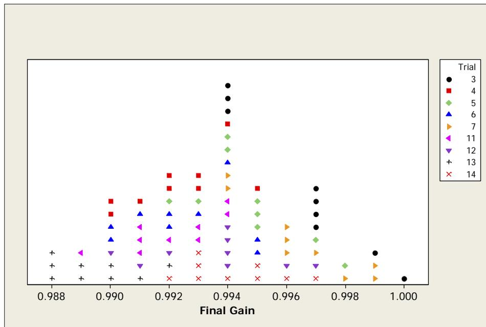
Fig. 2 Scatterplot of nine geophone calibration trials.
