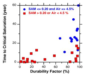
Figure 1 – Time to critical saturation as determined by the bucket test is shown versus the ASTM C 666 durability factor. Good agreement is shown between the two methods.
