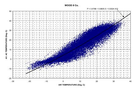
Figure 3 Air Temperature vs. Average AC Temperature (Wood 8 Co Station)
