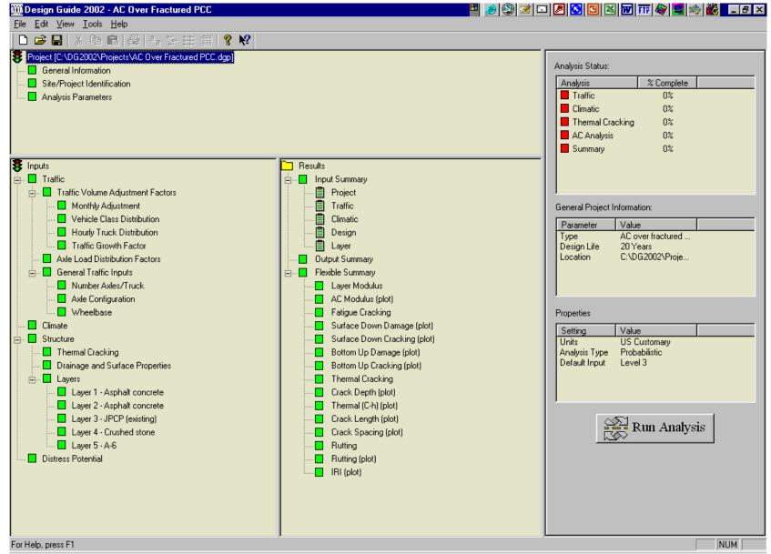
Figure A1. Example Input Summary Screen for 2002 Design Guide for AC overlay over Fractured PCC (Level 3 – Default Properties)
