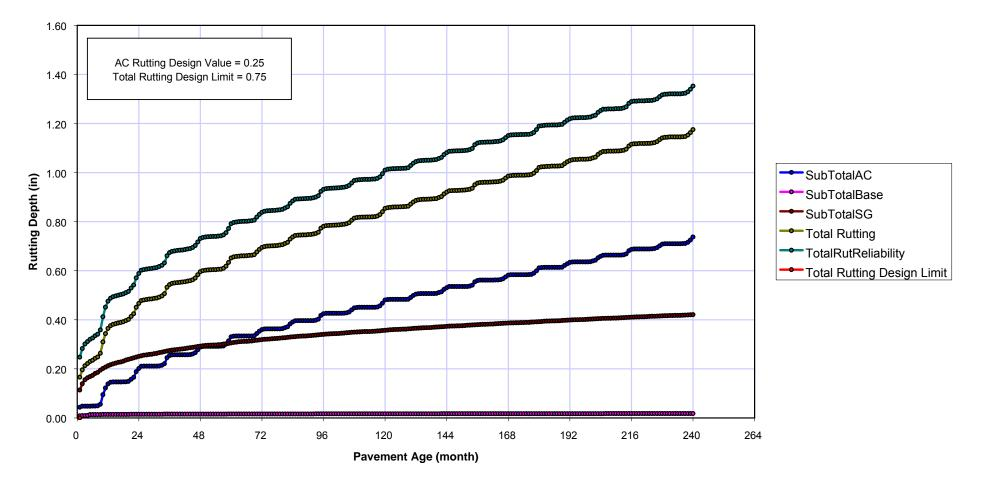
Figure A3. Example Output Permanent Deformation for 2002 Design Guide for AC overlay over Fractured PCC (Level 3 – Default Properties)
