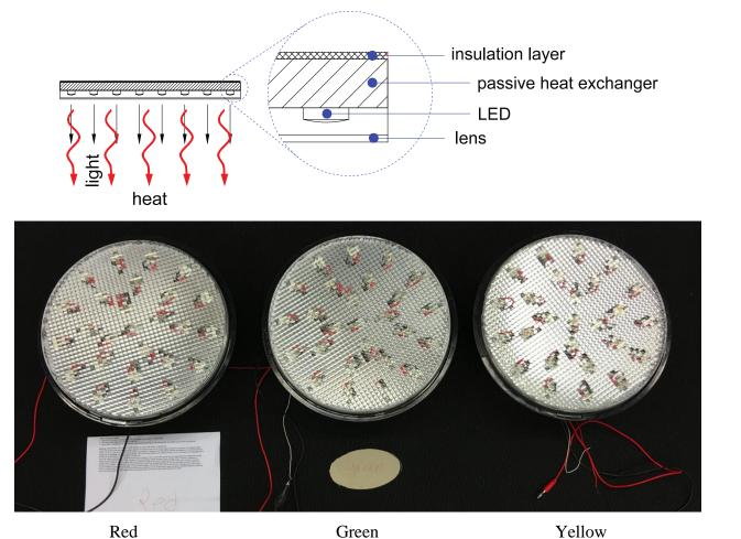
RedGreenYellowFigure 1Type 1 signal using the architecture of "Heat Arrangement of LED Arrays in Low Profile"(provisional patent filed in April 2016) to harvest both the light and the heat generated by the same LEDs via a<br/>mingled path for lighting and heating uses.
