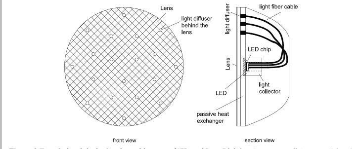
**Figure 2** Type 2 signal deploying the architecture of "Heated Lens Lighting Arrangement" (non-provisional patent application No. PCT/US14/53503) using a single high-power color LED module, a light collector and multiple light fibers.
