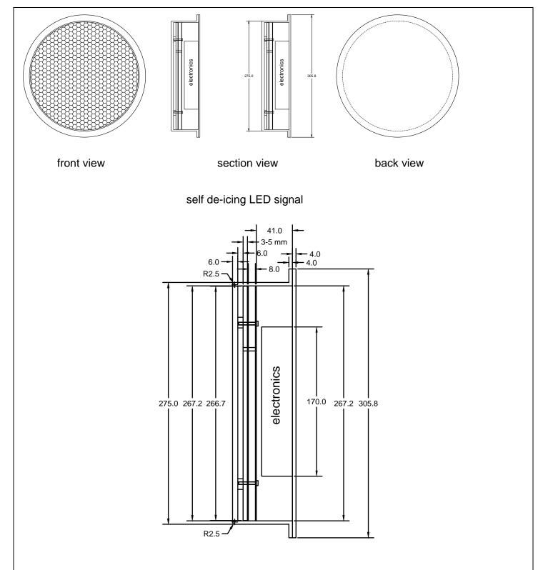
**Figure 3** The outlook of the finalized design of the self de-icing LED signal of Type 1, with approximate dimensions shown in the section view, in low profile (approx. only half of the thickness of current LED signals mounted in the field).
