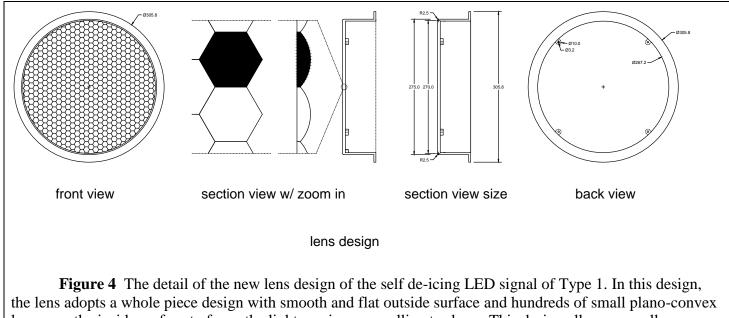
lenses on the inside surface to focus the light serving as a collimator lens. This design allows a small gap between the LEDs and the lens as small as <sup>1</sup>/<sub>4</sub> inch for enhanced thermal performance.
