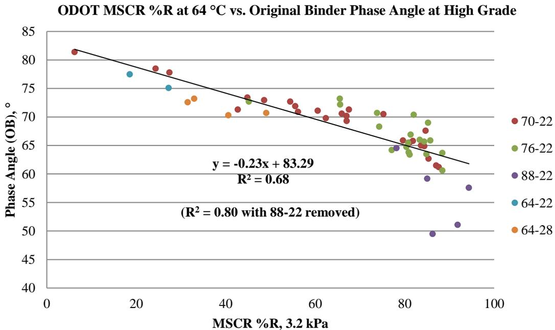
**Figure 5. ODOT MSCR %R at 64 C vs. Phase Angle at grade temperature.**
