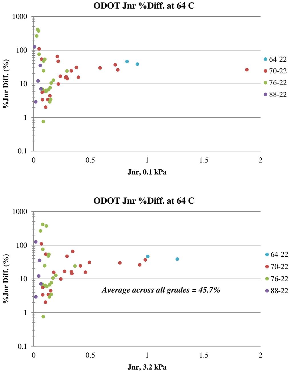
Figure 11. ODOT MSCR %Jnr Diff. vs. Jnr at two stress levels.
