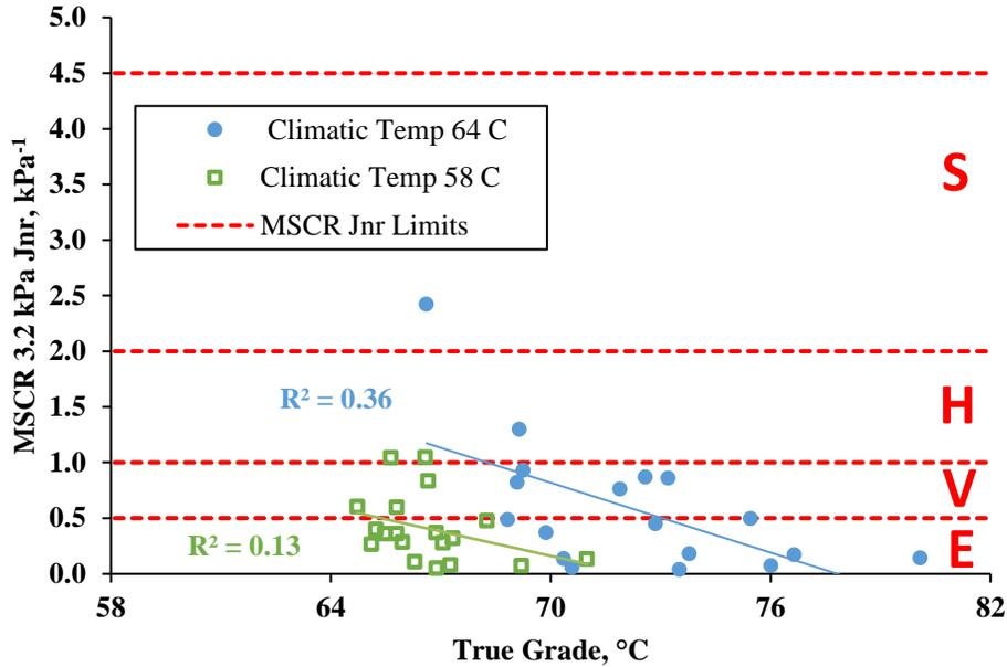
**Figure 12. Relationship between asphalt binder continuous grade and Jnr at 3.2 kPa.**
