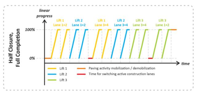
In this example, the first two lifts are paved in Lanes 1 and 2 before the first traffic switch. Subsequently, all lifts are paved in Lanes 3 and 4. After the second traffic-switch reverts the lanes available for construction back to the original configuration, the third and final lifts are paved in Lanes 1 and 2.
