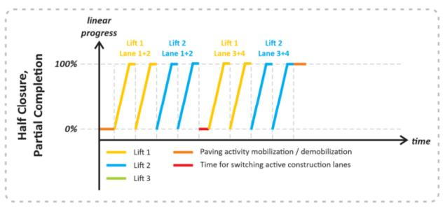
In this example again, the first two lifts are paved in Lanes 1 and 2 before the first traffic switch. Following this, the first two lifts are paved in Lanes 3 and 4 and the activity is concluded -- a second traffic-switch is unnecessary.
