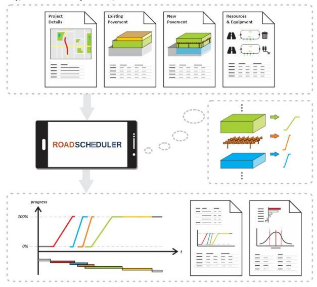
Starting with information you supply, Road Schedule interprets a pavement section as a set of material layers that each require some kind of construction activity, which in turn requires a
