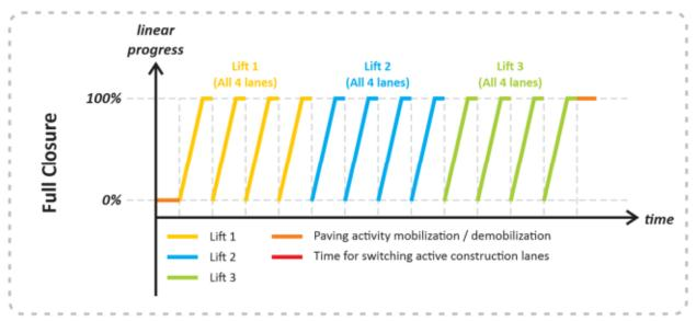
Each lift must have at least 1 additional adjacent lane available for a material supply truck. To represent this, Road Scheduler typically 'skips' lanes when it sequences lifts; for example, the lane sequence for the first lift may be 1, 3, 2, 4 so that the supply lanes are 2, 4, 1, 3 respectively. This pattern maximizes the amount of cooling time for a given lane and lift until a paver needs to begin the next lift layer.
