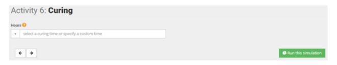
Incorporating curing in your simulation is important because concrete curing times can be long and limit when the roadway can be reopened to traffic. The curing time is compared to the paving activity and closure demobilization times to determine which activity is limiting.
