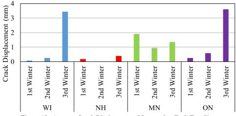
Figure 13. Average Crack Displacements Measured at Each Test Site
