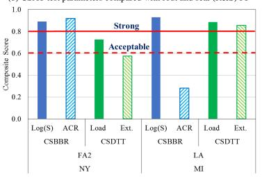
(c) CSBBR and CSDTT test parameters compared with clean and seal (C&S) PI Figure 34. Composite Score Correlating Test Parameters with PI for R&S and C&S Sections
