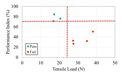
Figure 36. Sealants CSDTT Tensile Load vs. Performance Index
