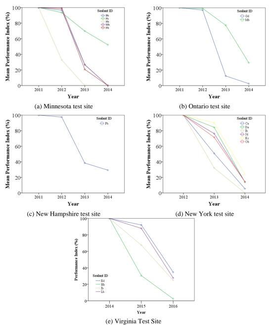
Figure 12. Overall Performance of Sealants for Clean and Seal Sections in Different Test Sites
