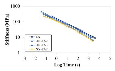
Figure 24. CSBBR Stiffness Master Curves Comparing Laboratory-Aged (LA) with Field-Aged (FAs) Samples for Sealant Da
