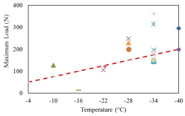
Figure 37. Selected Envelope for Sealant Peak Adhesion Load
