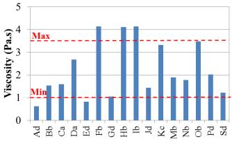
Figure 29. Viscosity Results for All Sealants
