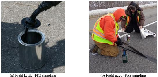
Kettle (FK) sampling (b) Field-aged (FA) sam Figure 7. Collection of Field-Aged Samples
