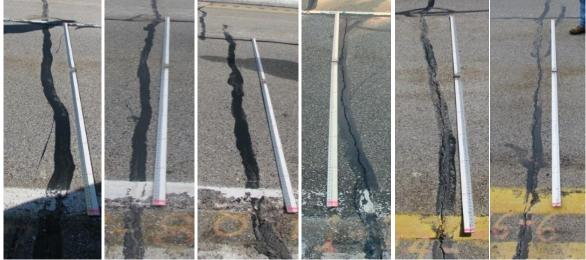
(a) Crack 5.7 (b) Crack 9.8 (c) Crack 8.7 (d) Crack 1.1 (e) Crack 14.9 (f) Crack 16.6 Figure 17. Sample Pictures for Sealants Field Performance in Michigan Test Site
