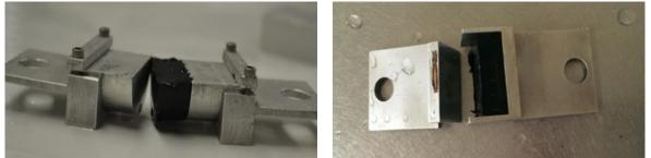
(a) CSAT (b) Modified Adhesion Test Figure 10. Specimen Configuration for Current and Modified Tensile Adhesion Tests
