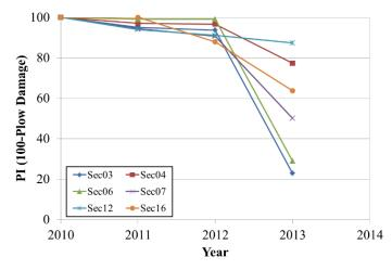
Figure 18. PI of Selected Sealants Based on Plow Abrasion (%OBF: Overband Failure)
