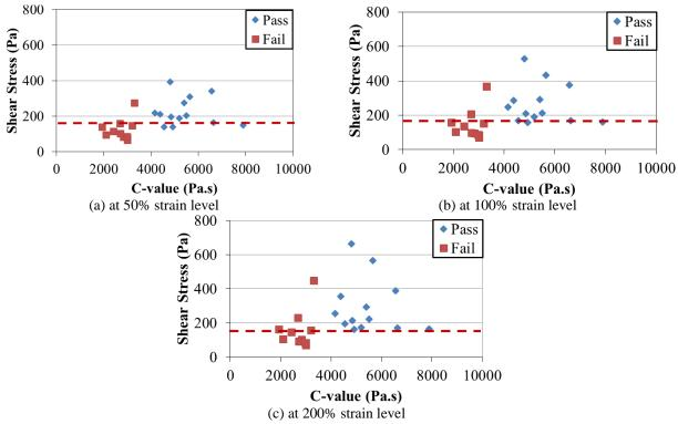
Figure 27. Shear Stress Threshold for Yield Testing at Different Strain Levels
