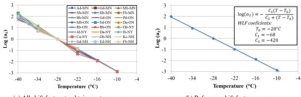
(a) All shift factors to obtain master curves **Figure 35. Shift Factors for All Field-Aged Sealants to Obtain Master Curve at -28°C**
