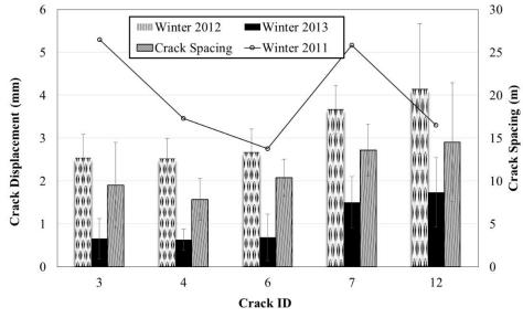
Figure 20. Average Crack Displacement and Spacing
