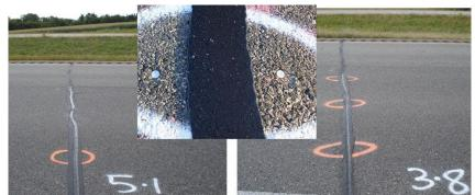
Figure 3. Crack Displacement Pins: Single-Point to Measure Only Right Wheel Path (left) and Three-Point to Measure Both Wheel Path and Middle of the Lane (right)
