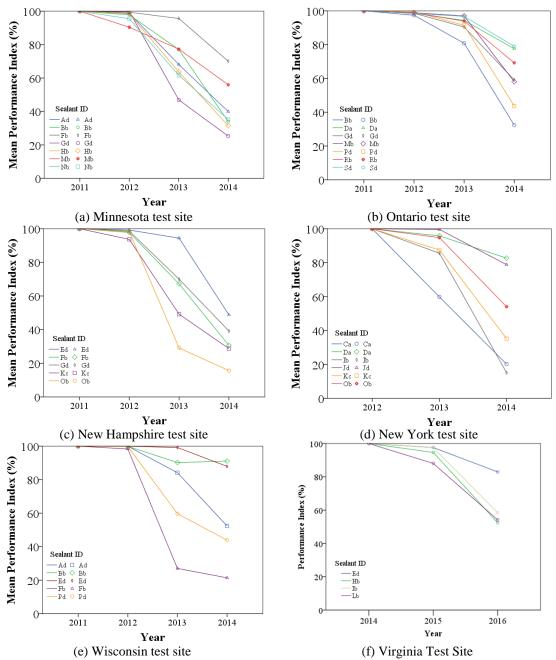
Figure 11. Overall Performance of Sealants for Rout and Seal Sections in Different Test Sites
