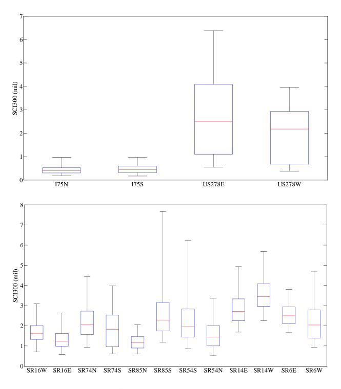
Figure 8. SCI300 box plot of tested roads in 2014.
