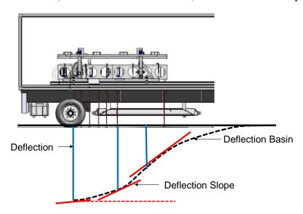
Figure 3. Relationship between the deflection basin, deflection, and deflection slope (modified from Krarup 2012).
