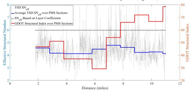
Figure 17 Comparison of Effective Structural Number on SR74S calculated from TSD measurements collected in 2015 and GDOT Structural Index
