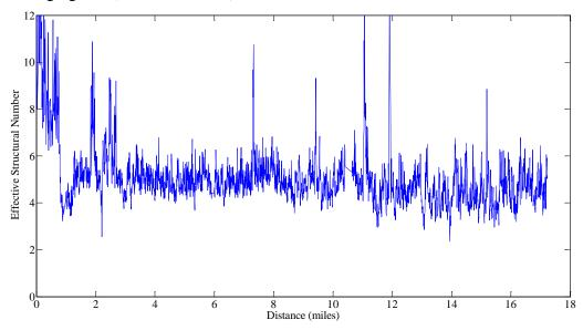
Figure 16 Effective Structural Number on SR16E calculated from measurements collected in 2015
