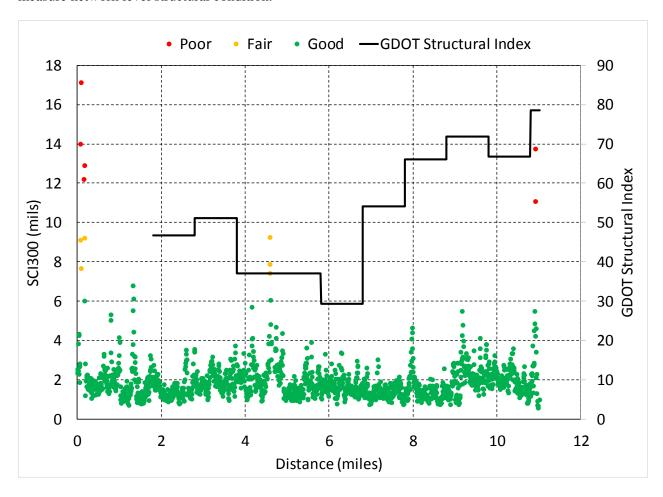
Figure 12 Comparison on SR74 in Fayette County between TSD SCI300 measured in 2015 and Structural Index obtained from surface distresses (<a href="https://goo.gl/maps/azJkphpKdBo">https://goo.gl/maps/azJkphpKdBo</a>)
