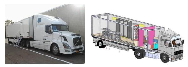
Figure 1. TSD used during testing (left) and computer-generated schematic (right) (Krarup, 2012).
