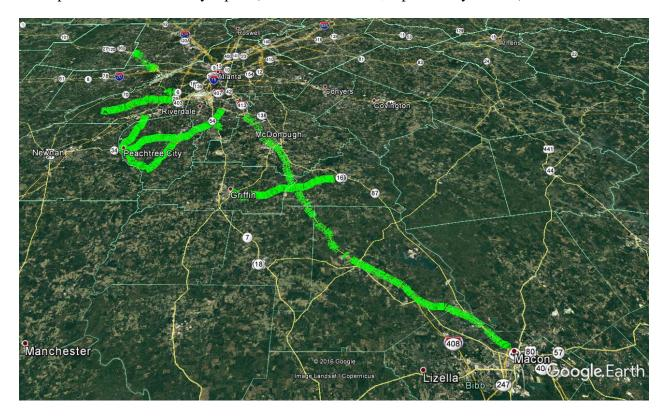
Figure 5. Color-coded estimated structural condition of tested roads in 2014 with Good (green), Fair (yellow), and Poor (red) ratings (© 2016 Google Image Landsat / Copernicus).
