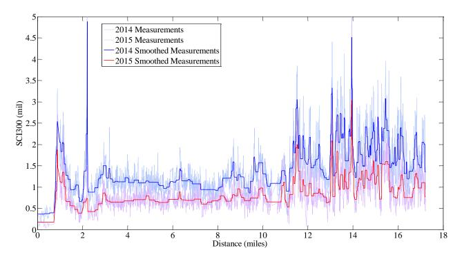
Figure 10. Temperature corrected repeated TSD tests (SCI300) on SR16E (https://goo.gl/maps/2LXJWXbGQLE2)
