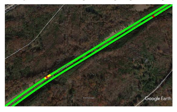
Figure 7. Detail example of estimate pavement structural condition on SR14 south east of Atlant tested in 2015 (© 2016 Google Image Landsat / Copernicus).
