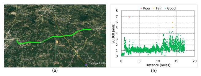
Figure 13. Identified Strong (green) and Weak (red) sections on SR16 east based on thresholds obtained from Table 2: (a) Google Earth plot (© 2016 Google Image Landsat / Copernicus); (b) figure plot
