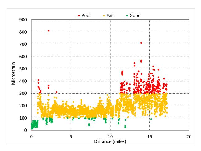
Figure 18. Estimated tensile strain at bottom of asphalt layer on SR16 east.
