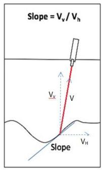
Figure 2. Schematic of the measurement principle of the TSD (Krarup 2012 and modified from Flintsch et al. 2013).
