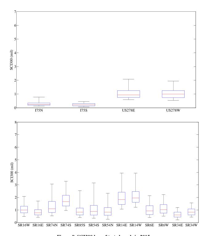
Figure 9. SCI300 box of tested roads in 2015.
