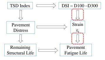
Figure 19. Link between DSI and estimated pavement fatigue life.
