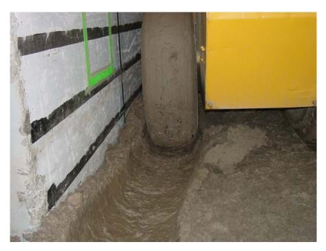
Figure 19. Unstable soil behavior with gravimetric moisture contents between 27 and 35 percent.
