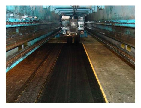
Figure 25b. Test Window 712c6 at the end of HVS traffic
