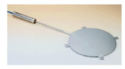
Figure 11. Large Geokon® stress cell used in the base course.
