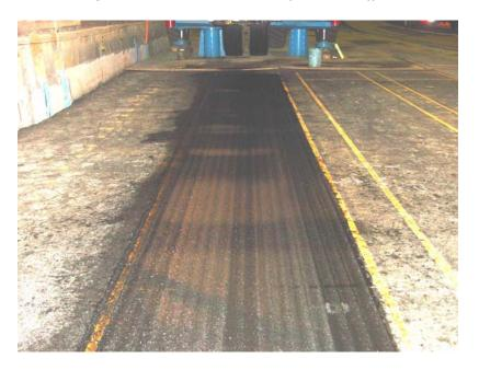
Figure 20b. Test Window 712c1 at the end of HVS traffic.
